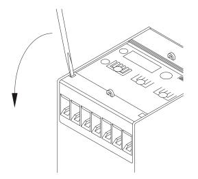
3. Carefully remove the battery by means of a fully isolated screw driver out of the plug terminals. Replace the battery. Ensure the correct polarity.
