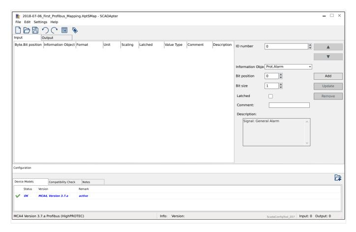
The mapping table is distributed over two tabs, "Input" and "Output". The data-points listed in "Output" will be sent by the Master to the Slave (and the slave, in our case, is the protection device), and the data-points listed in "Input" will be sent by the Slave to the Master.
