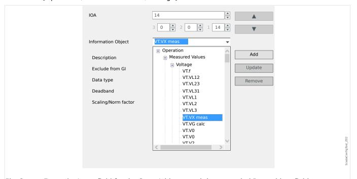
Fig. 3: Example: Input field for the Start Address, and the expanded Data object field.
