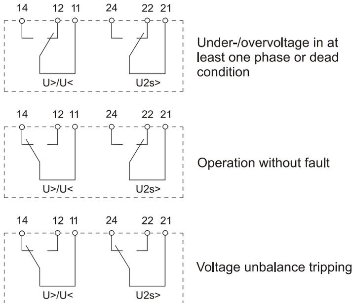
Figure 2.3: Contact positions of the output relays
