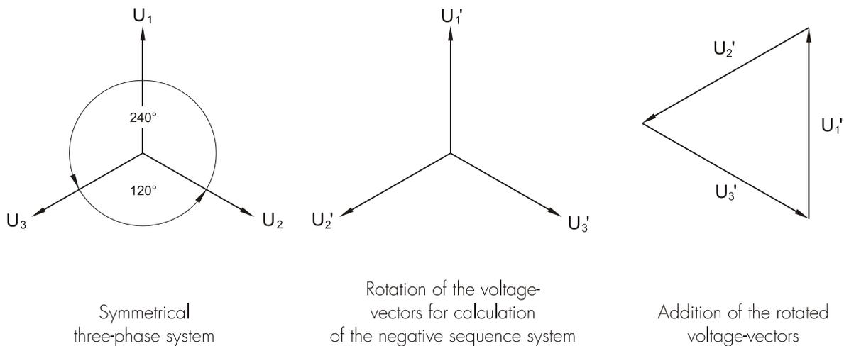
Figure 3.1: Symmetrical three-phase system
