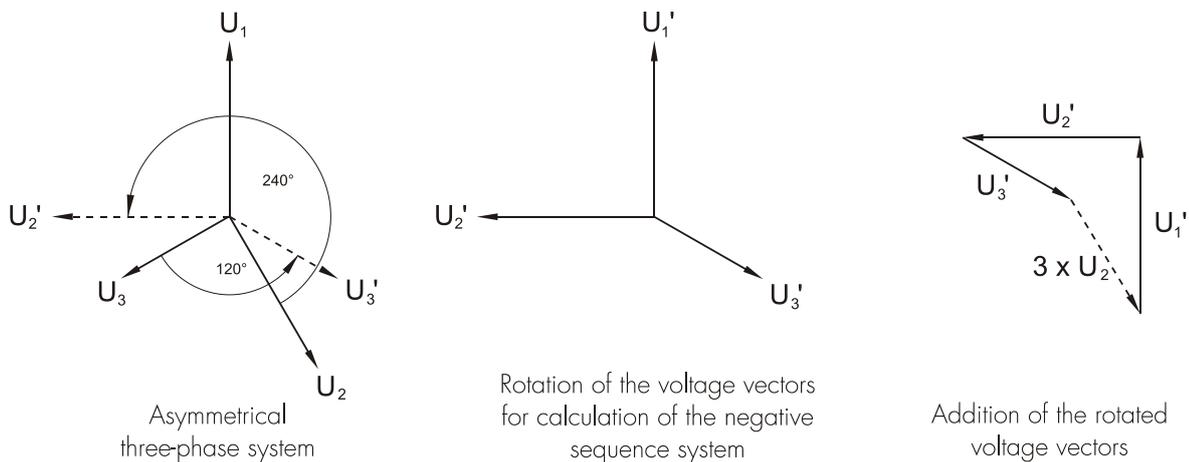
Figure 3.2: Asymmetrical three-phase system
