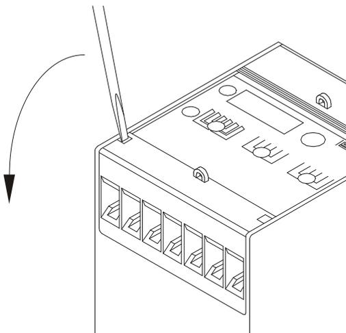
Figure 4.2: How to open the transparent cover
