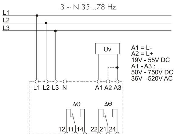
Figure 2.2: Connection three-wire system  $\Delta$
