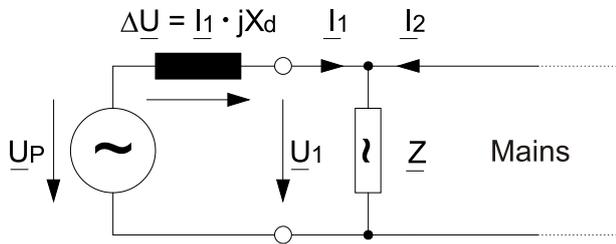
Figure 3.1: Equivalent circuit of synchronous generator in parallel with the mains
