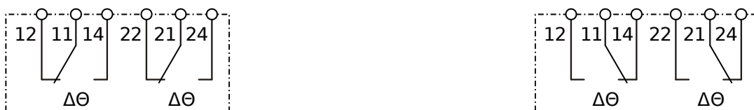
Figure 2.2: Contact positions of the output relays – left: Operation without fault or dead condition, right: Contact positions after tripping.
