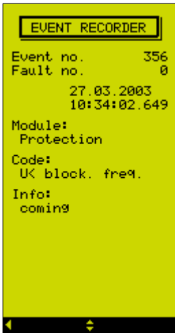
Figure 5.6: Screenshot of the information to be called up out of the "EVENT RECORDER"
