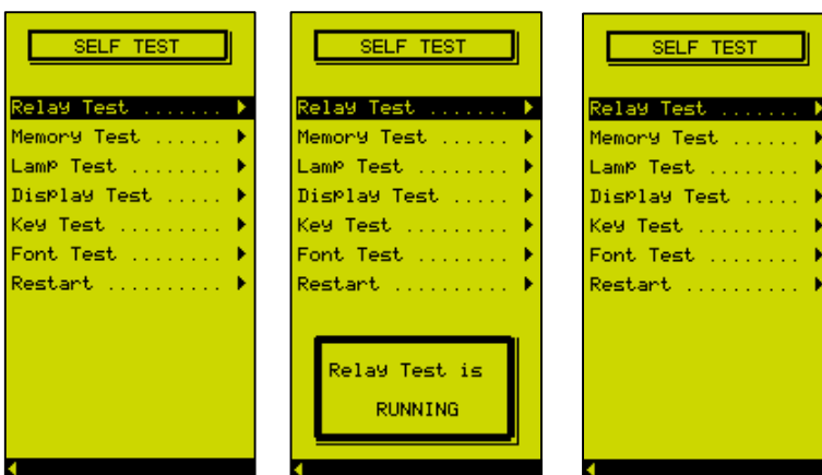
Figure 5.100: Implementation of the " relay test "
