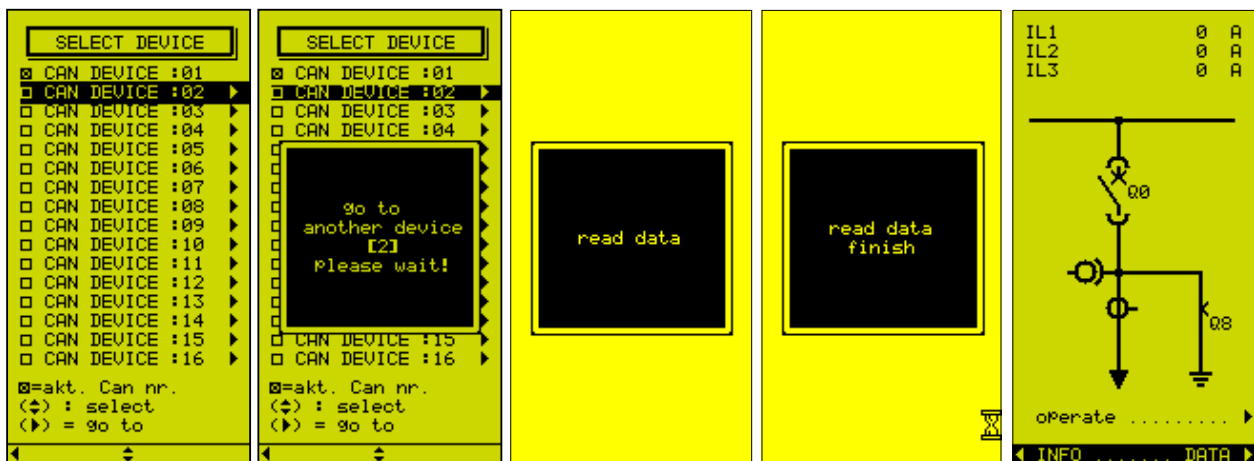
Figure 5.82 Logging into another CSP-system via the "Select device"-menu (Variant 2)
