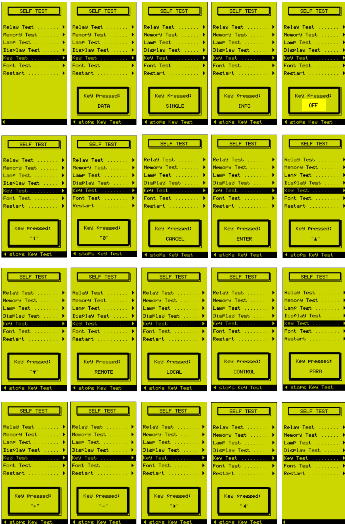
Figure 5.77: Execution of the "keyboard test"
