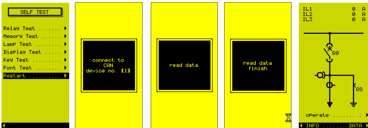
Figure 5.79: Execution of the "restart"
