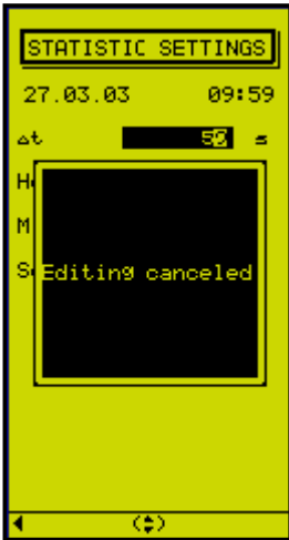
Figure 3.20: Pop-up windows e.g. at setting of undefined mode of operations
