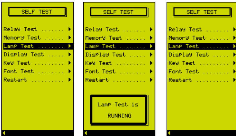
Figure 5.75: Execution of the "lamp test"
