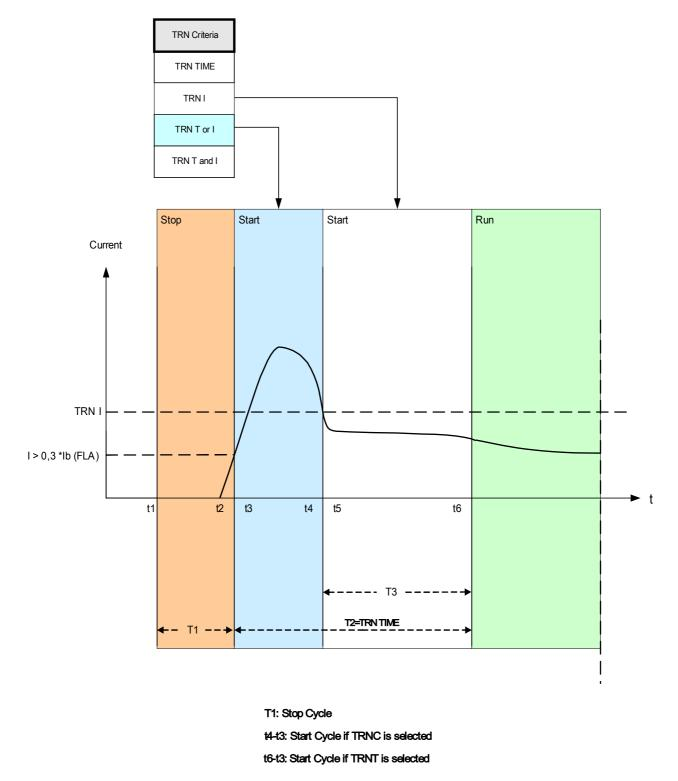
The Start Control Module drawing shows an example of how the protective device reacts to a normal operatingcycle current profile. Initially, the motor is stopped and the current is zero. As long as the protective device is not in a »trip« state, it permits contactor energization by closing its trip contact in series with the contactor. The contactor
