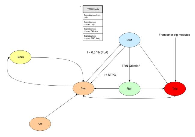
The basic motor operation states can be classified as four states that include:
