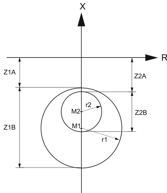
Figure 4.1: Tripping zones of the underimpedance elements
