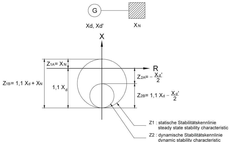
Figure 5.1: Setting adapted to the steady state and dynamic stability characteristic
