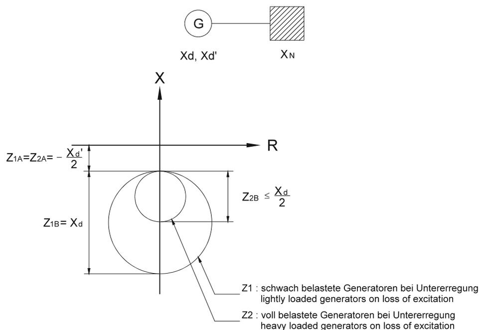
Figure 5.2: Selective protection with any generator load
