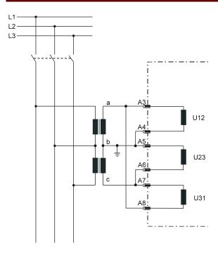
Figure 3.3: Voltage transformer in V-connection
