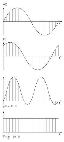
Figure 4.1: Power measurement
