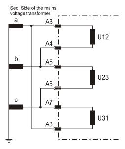
Figure 5.2: Input transformers in delta-connection (MRP2-3)
