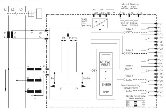
Figure 3.1: Connection diagram MRP2-1 and MRP2-R1 (Star-/Delta adjustment has to be set to DELTA)
