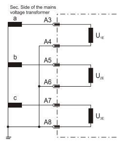
Figure 5.3: Input transformers in star-connection (MRP2-3)
