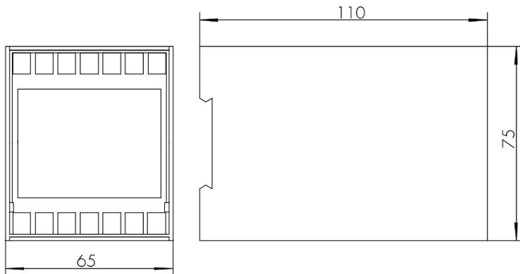
Figure 2: Dimensional drawing of BUA1
