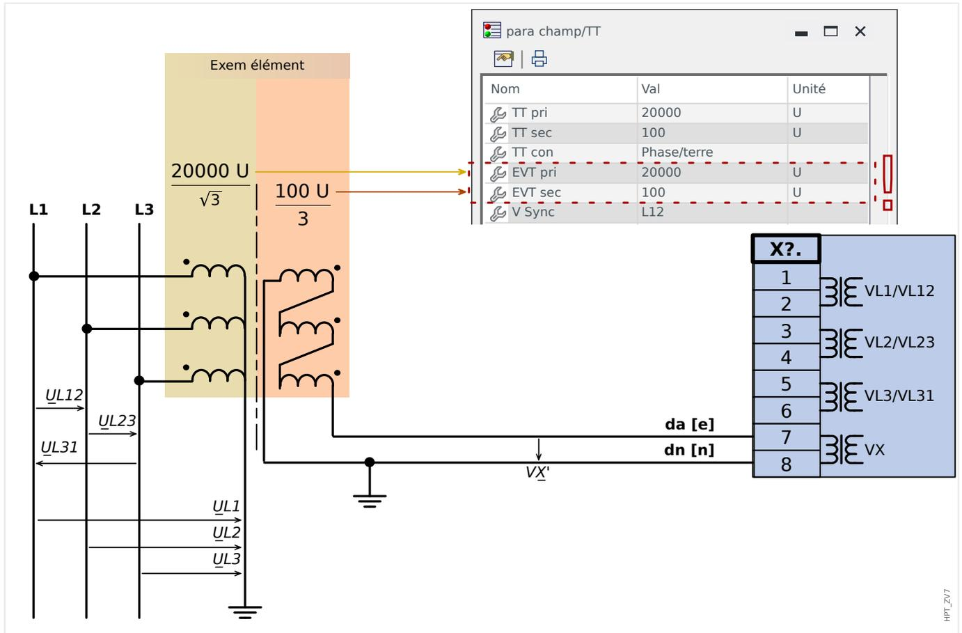
After the voltage inputs have been connected correctly the residual voltage is measured with the following setting:
