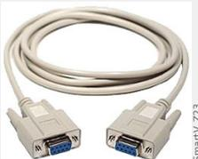
A white null-modem cable with two RS-232 connectors. The label 'SmartV_Z23' is visible at the bottom right of the image. |
