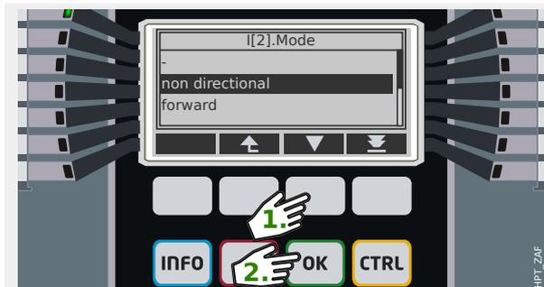
Press "▼" (Down) repeatedly again, until the required value, for instance: "non directional", is highlighted.
