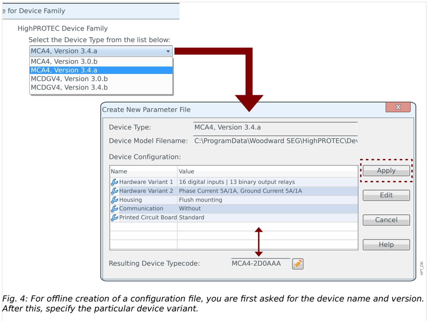
Fig. 4: For offline creation of a configuration file, you are first asked for the device name and version. After this, specify the particular device variant.
