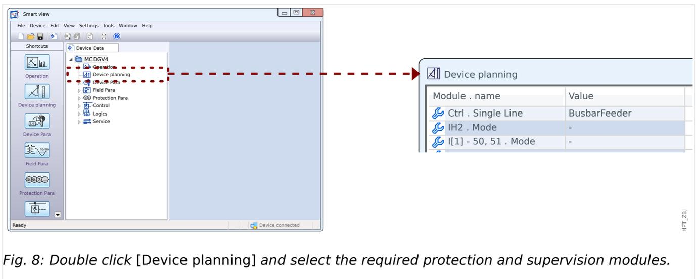
Fig. 8: Double click [Device planning] and select the required protection and supervision modules.
