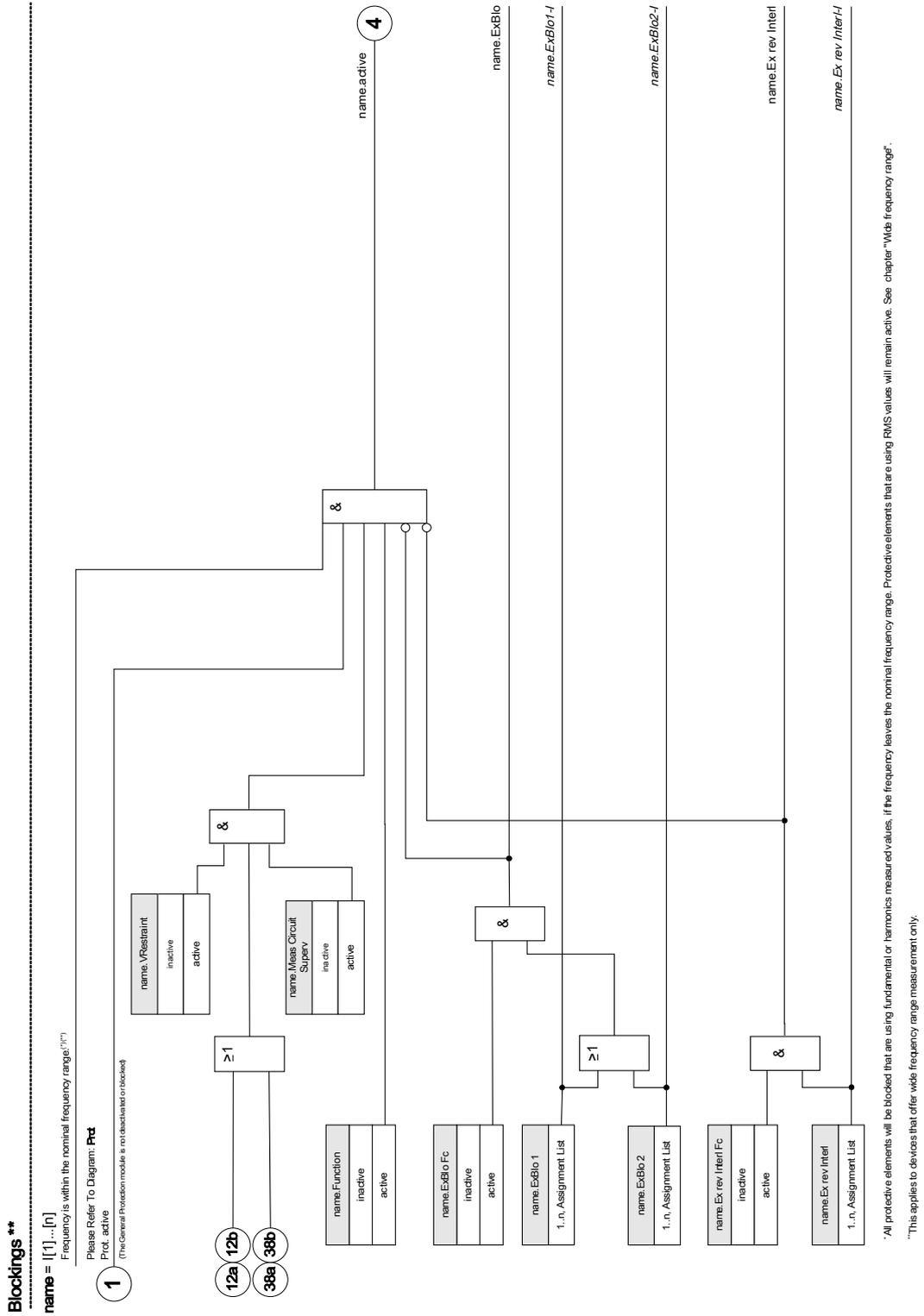
Earth current protective functions cannot only be blocked permanently (»function = inactive«) or temporarily by any blocking signal from the »assignment list«, but also by »reverse Interlocking«.
