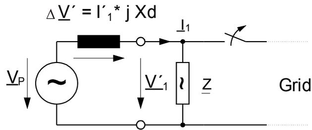
In case of mains failure or auto reclosing the generator suddenly feeds a very high consumer load. The rotor displacement angle is decreased repeatedly and the voltage vector  $V_1$  changes its direction ( $V_1'$ ).
