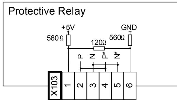
Electro-mechanical assignment Type 1 (see wiring diagram)
