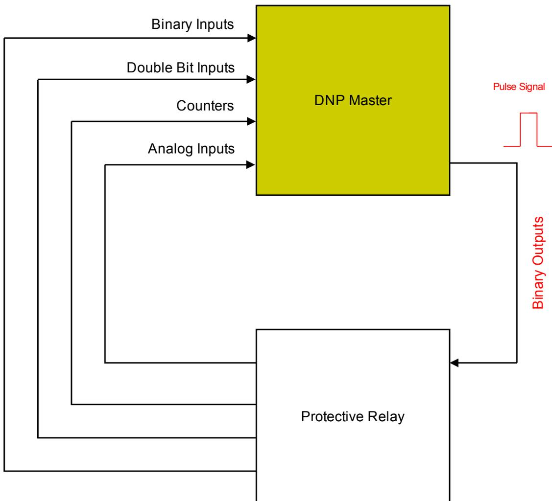
Please try to avoid gaps that will slow down the performance of the DNP communication. That means do not leave unused inputs / outputs in between used inputs / outputs (e.g. Do not use Binary Output 1 and 3 when 2 is unused).
