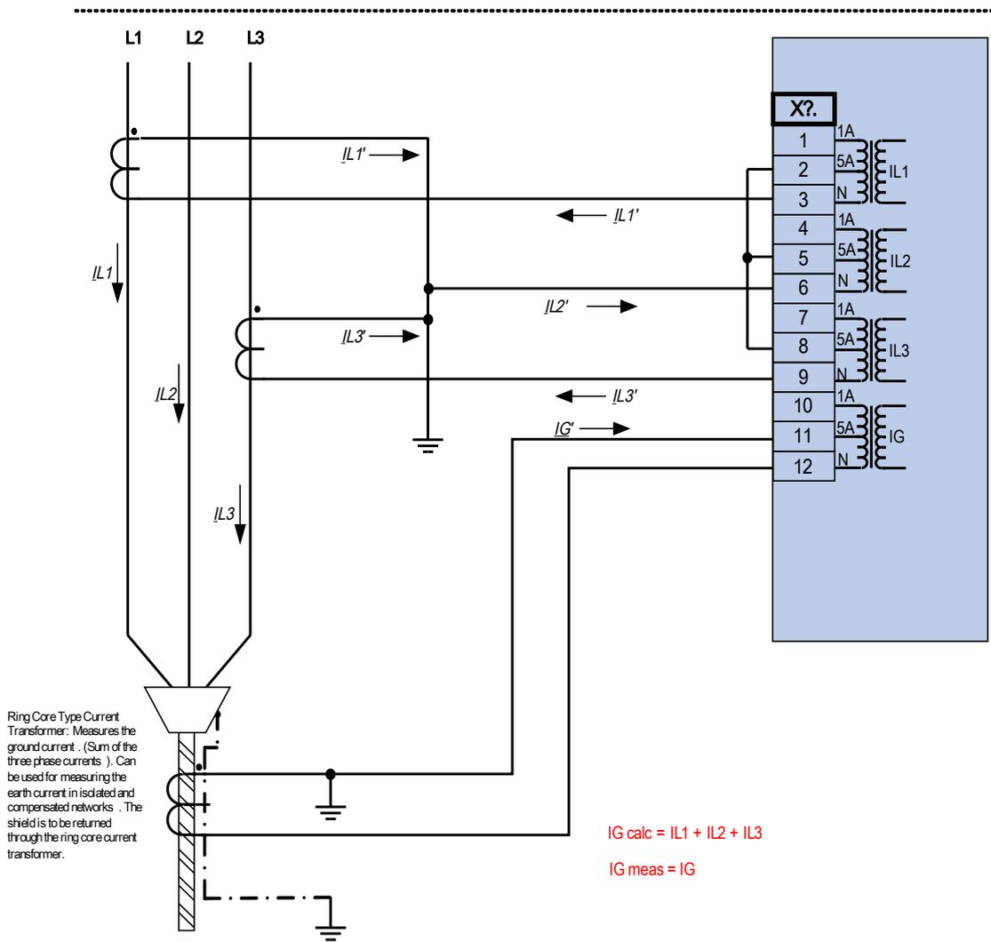
Two phase current measurement (Open Delta); In secondary = 5 A.
