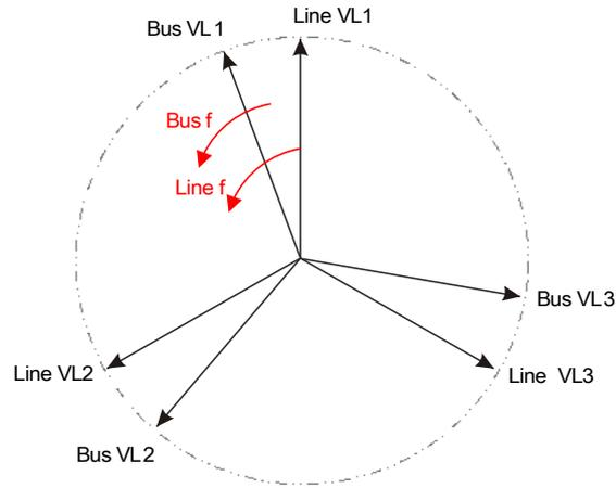
If the generator frequency  $f_{\text{Bus}}$  is not equal to the mains frequency  $f_{\text{Line}}$ , it results in a slip frequency  $\Delta F = |f_{\text{Bus}} - f_{\text{Line}}|$  between the two system frequencies.
