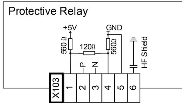
*Electro-mechanical assignment Type 2 (see wiring diagram)*
