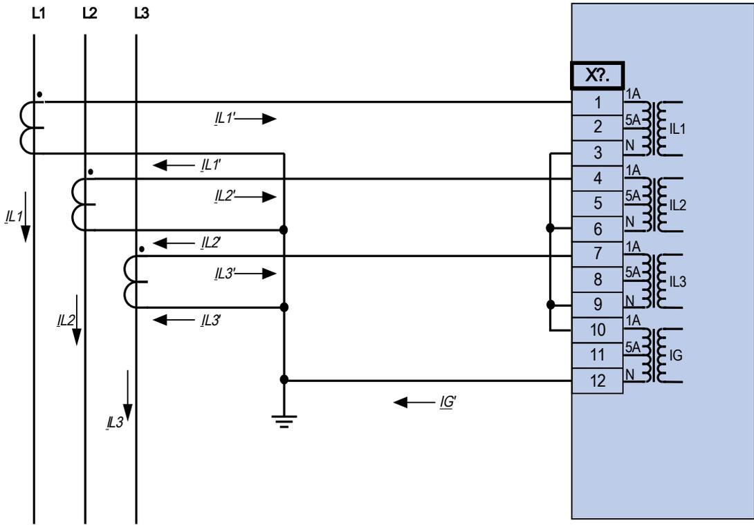
Three phase current measurement;  $I_n$  secondary = 1 A.
