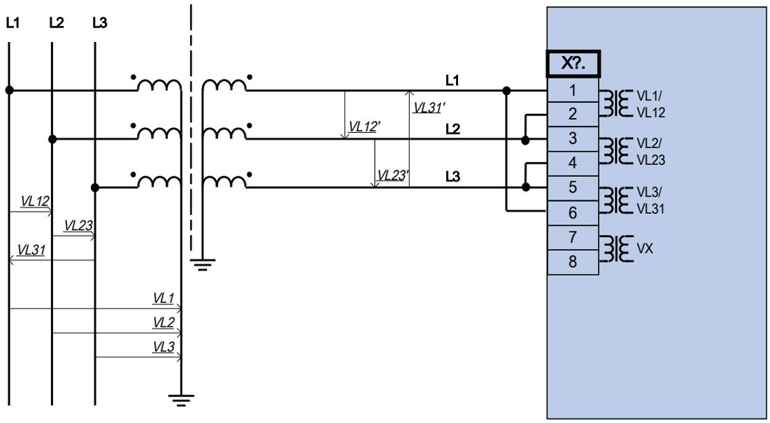
Three-phase voltage measurement - wiring of the measurement inputs: "delta-connection"
