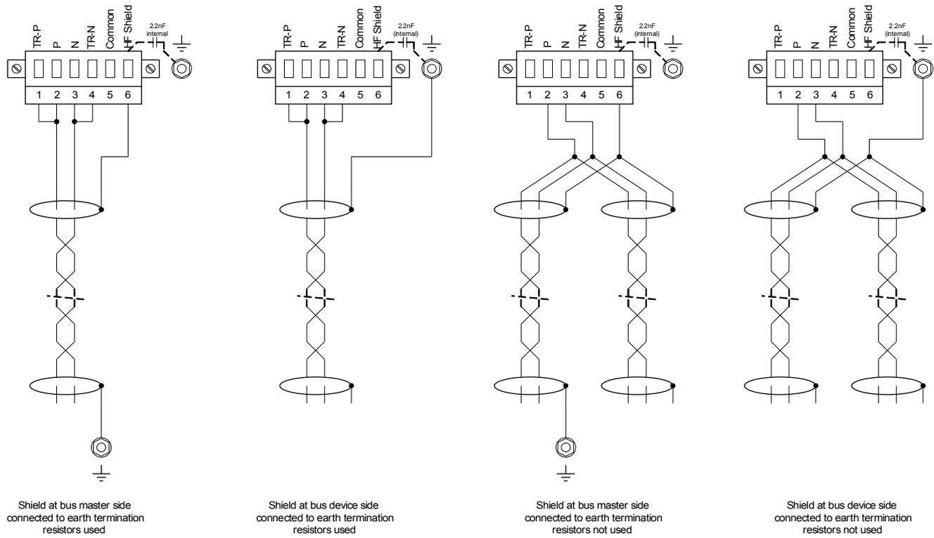
Type 2 Shielding Options (3-wire + Shield)
