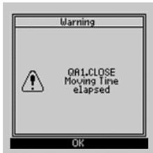
Notice: For the case, the switchgear does not reach the new end position within the set supervision time the following Warning appears on the display.
