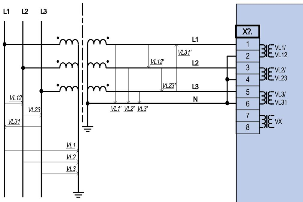
Three-phase voltage measurement - wiring of the measurement inputs : "star-connection"
