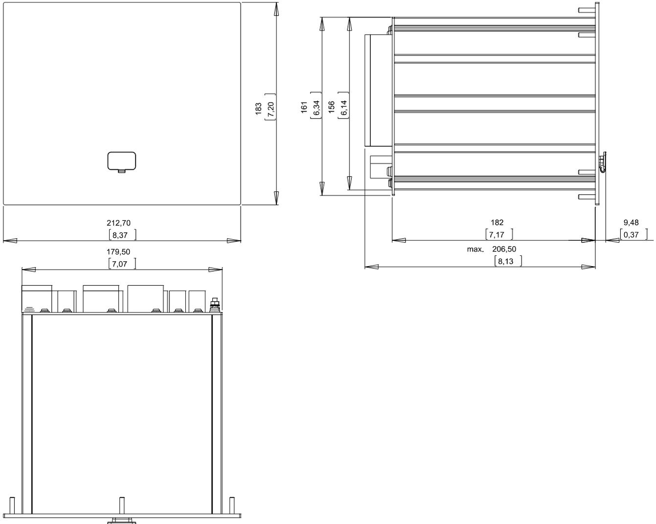
3-Side-View B2 Housing (Devices with 8 Softkeys)
