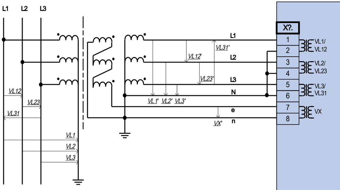
Three-phase voltage measurement - wiring of the measurement inputs: "star-connection"
