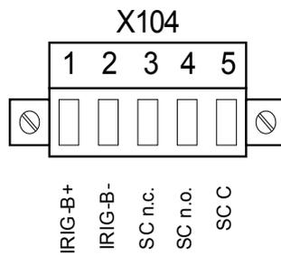
The *System-OK contact (SC relay)* cannot be configured. The system contact is a changeover contact that picks up when the device is free from internal faults. While the device is booting up, the *System OK relay (SC)* remains dropped-off (unenergized). As soon as the system is properly started (and protection is active), the System Contact picks up and the assigned LED is activated accordingly (please refer to the Self Supervision chapter).
