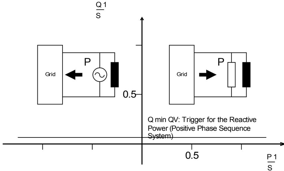
A minimum current supervision ( $I_1$ ) in the positive phase sequence system prevents a hyperfunction of the reactive-power supervision at lower power levels.
