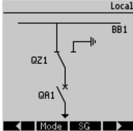
This switchgear is a combination of a disconnecter and an earthing switch. This Switch switches between the »ON-Position« (e.g. Busbar) and the »Earthing-Position«.
