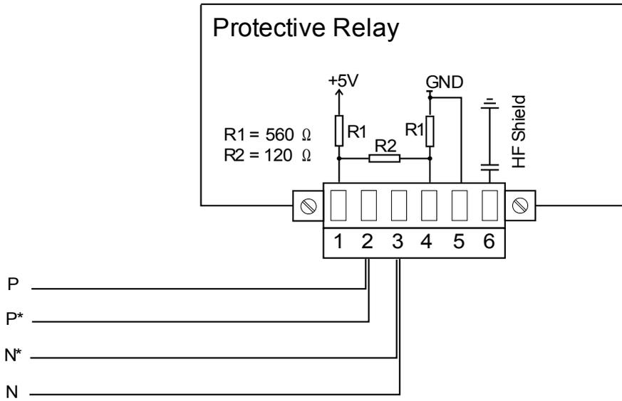
Type 2 Wiring example, Device at the End of the BUS (using the integrated Terminal Resistor)
