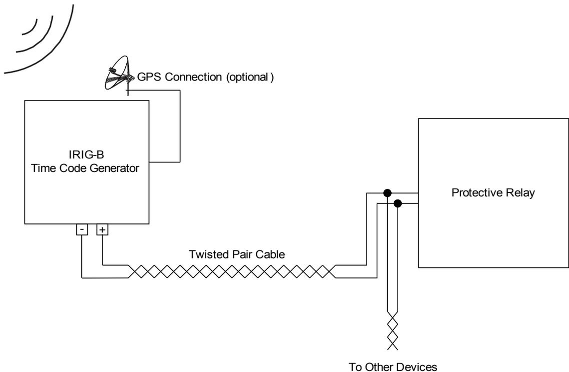
The location of the IRIG-B interface depends to the device type. Please refer to the wiring diagram supplied with the protective device.
