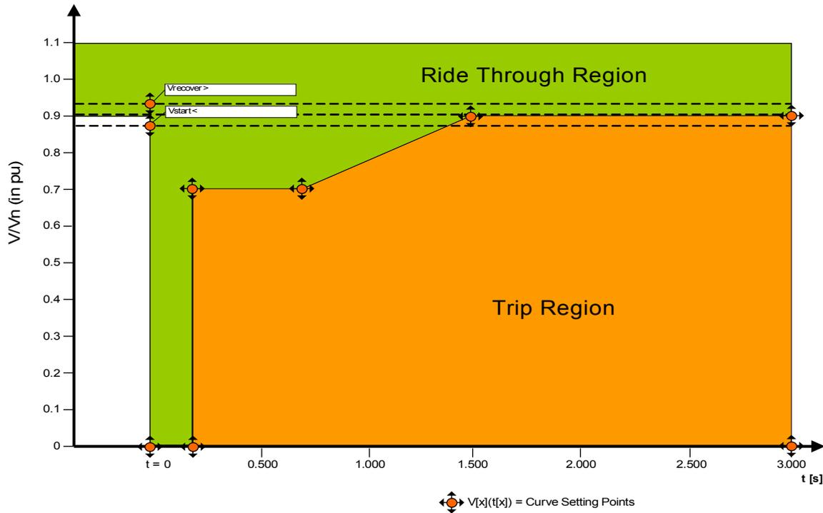
The LVRT element will change into standby again as soon as the system voltage recovers: That means, the voltage has risen above the preset recover voltage » *Vrecover*«.
