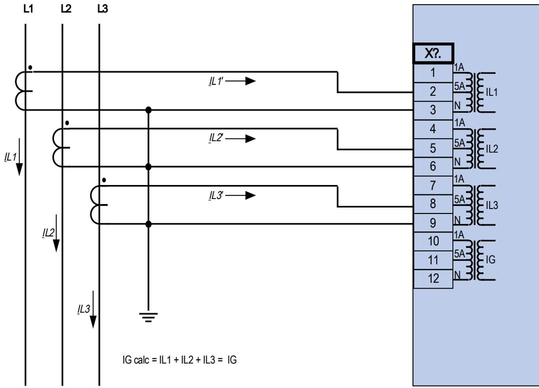
Three phase current measurement; In secondary = 5 A.
