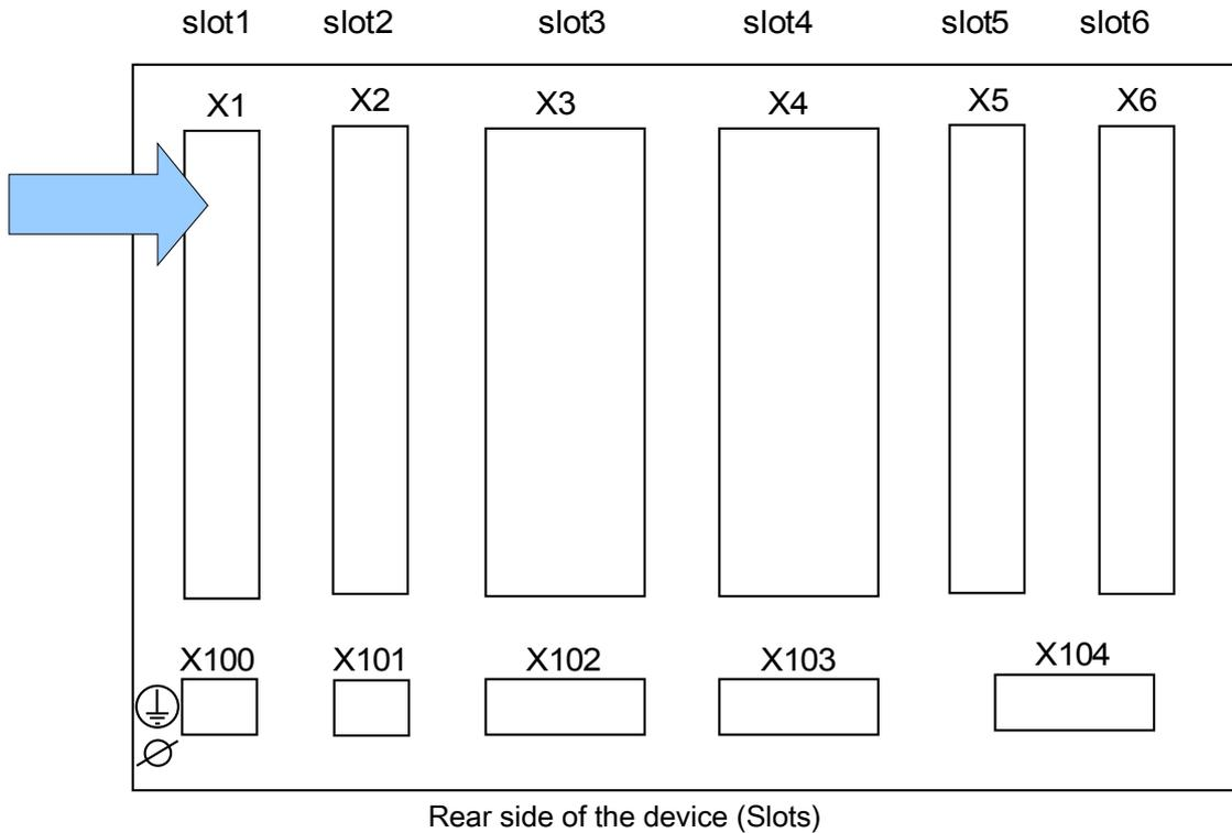
The type of power supply card and the number of digital inputs on it used in this slot is dependent on the ordered device type. The different variants have a different scope of functions.
