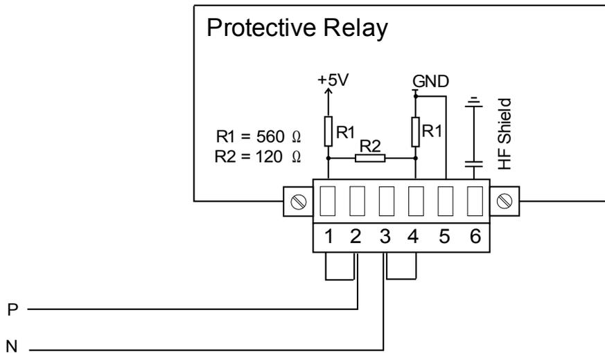
Type 2 Shielding Options (2-wire + Shield)
