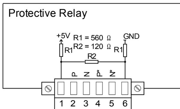
**NOTICE** The Modbus® / IEC 60870-5-103 connection cable must be shielded. The shielding has to be fixed at the screw which is marked with the ground symbol at the rear side of the device.
