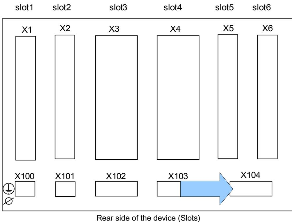
This comprises the IRIG-B00X and the System contact (Supervision Contact).
