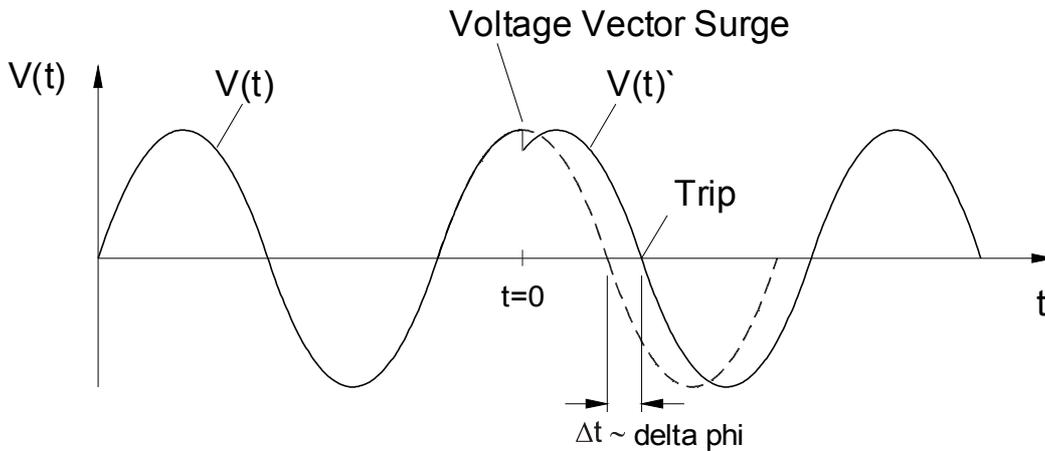
As shown in the voltage/time diagram the instantaneous value of the voltage jumps to another value and the phase position changes. This is called phase or vector surge.
