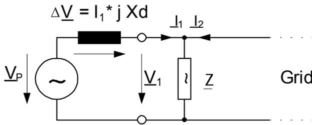
Voltage vectors at mains parallel operation.
