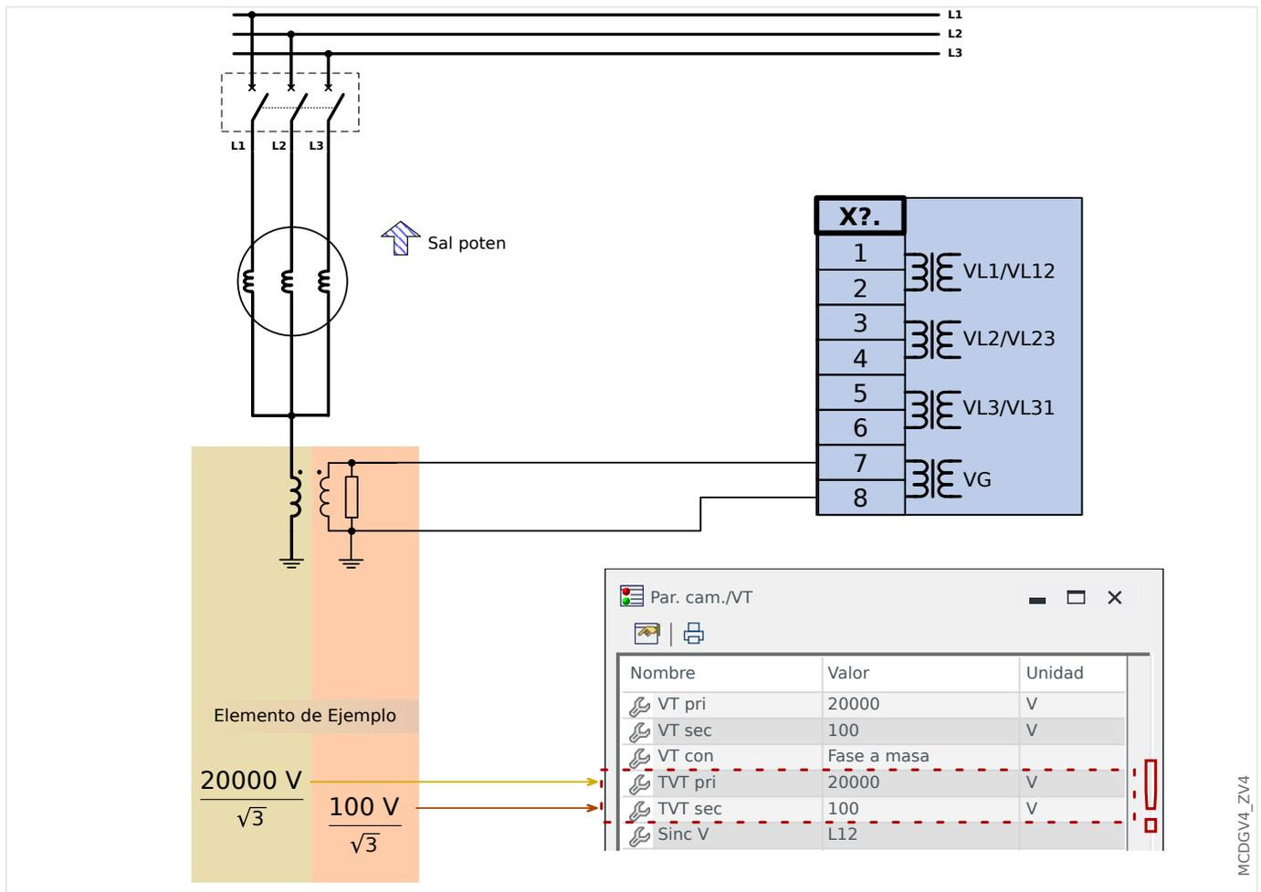
After the voltage inputs have been connected correctly the residual voltage is measured with the following setting:
