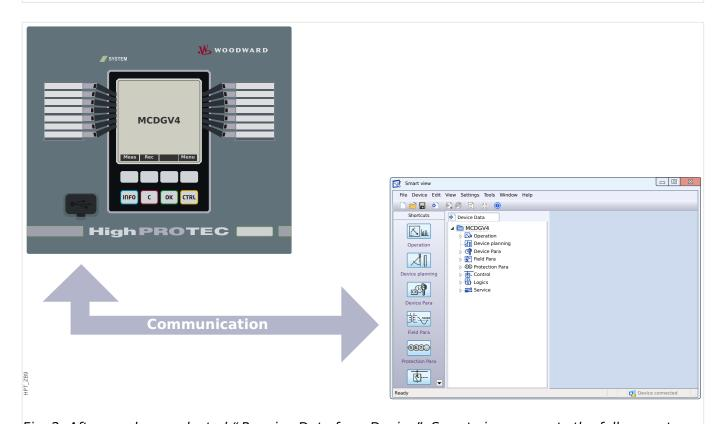
Fig. 2: After you have selected "Receive Data from Device", Smart view presents the full menu tree.
