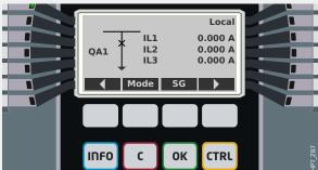
The new position of the switchgear device is shown on the display (as soon as it has been reached according to the feedback of the position indication, or after the configured switching time has elapsed).
