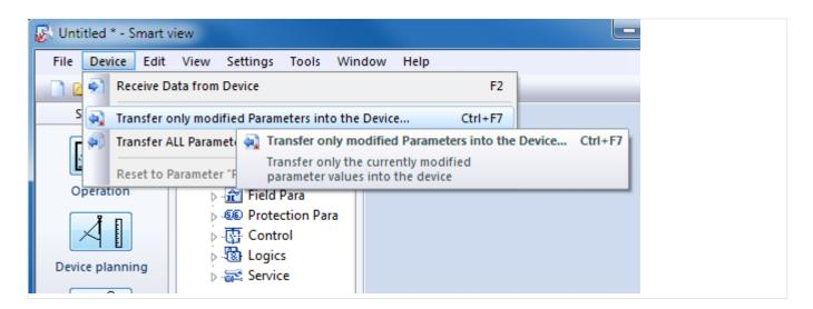
• This transfer of the changes involves entering the password of the protective device. After it has been correctly entered the changes are sent to the device (and the device activates the new settings).
