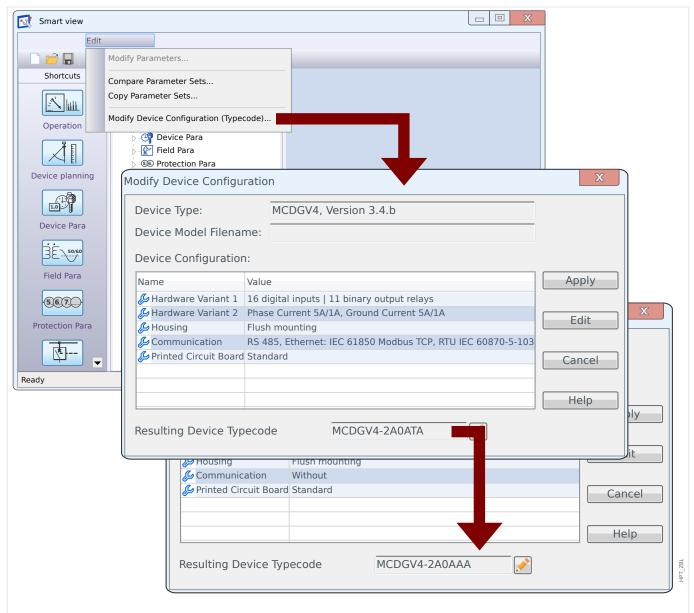
Fig. 5: Converting a configuration file from "MCDGV4-2A0ATA" to "MCDGV4-2A0AAA".
