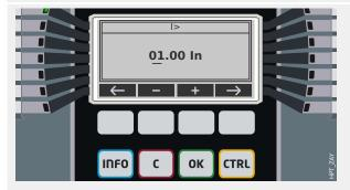
Since this is a number value you see a special numeric editing dialog: A flashing cursor is underlining one of the digits, and with the Softkeys "+" or "-" you can increase or decrease the digit, respectively. The Softkeys "←" (Left) or "→" (Right) move the cursor one decimal place to the left or right, respectively.
