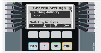
As an example, we want to execute a switching operation now. Therefore we check the switching authority first and enter the menu branch [Control / General Settings] (e.g. by pressing the Softkey "Mode").
