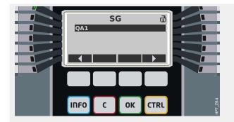
When the single-line is being displayed, the Softkey "SG" takes you to a screen that lists all connected switchgear devices.
