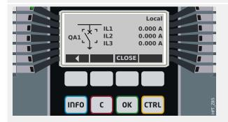
When the single-line is being displayed, the Softkey "▶" (Enter) takes you to an enhanced single line (after you have entered the password for access level "Control-Lv1"). The switchgear device is highlighted by small markers (and in case of several implemented switchgear devices, the Softkey "Select" is visible, which allows you to select another one).
