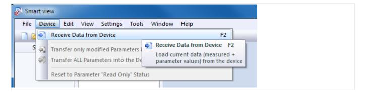
• Smart view establishes a connection with the protective device, reads data from it and displays these values in form of a tree structure.
