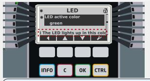
The **information** token "**i**" has already been mentioned in "Parameter Changes – "OK" key". It appears as part of a setting dialog (on the device display in a dedicated line of text, directly above the Softkey assignments, or as a text frame within a *Smart view* setting dialog window). It indicates the detailed description of the parameter in question.
