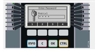
Similar to the modification of a setting (see Parameter Changes – "OK" key") you are asked for the password (this time, however, level "Prot-Lv1" is sufficient).
