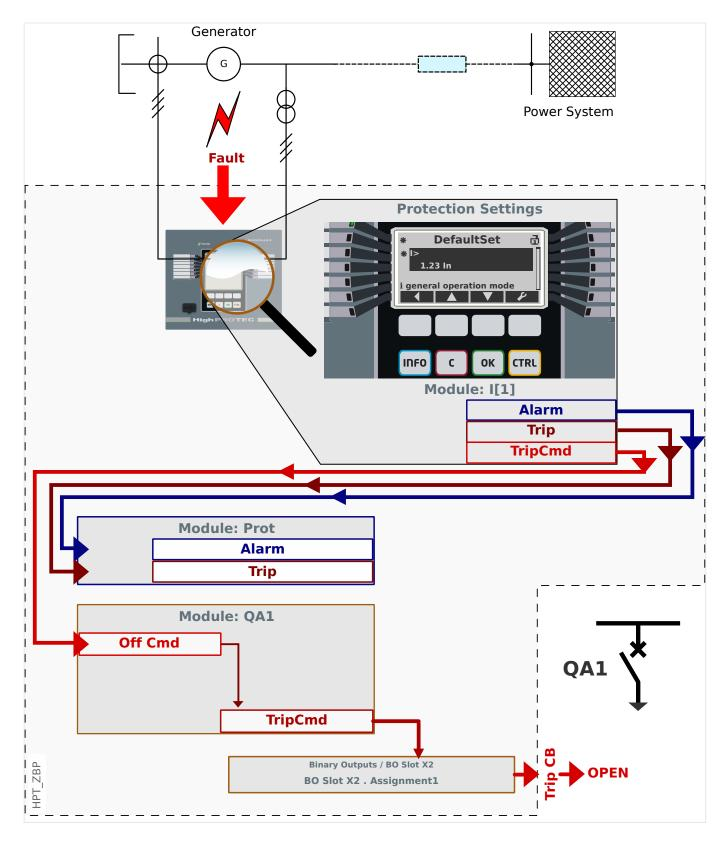
Let us take a simple, non-directional phase overcurrent protection as an example (see diagram above), e. g. the module I[1].
