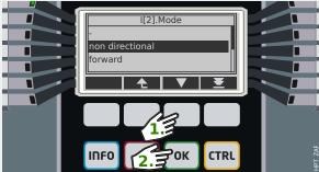
Press "▼" (Down) repeatedly again, until the required value, for instance: "non directional", is highlighted.
