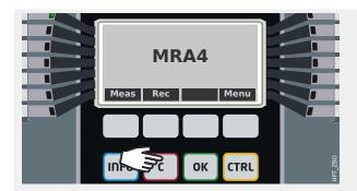
The [Acknowledge] menu allows to "acknowledge" (i. e. reset) latched signals, output relays and/or trip commands. This menu branch can be accessed the usual way, but there is also a short-cut: The "C" key takes you there directly.
