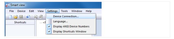
• Select "Ethernet Connection" in the dialog. Then enter the TCP/IP address of the protective device into the input field.
