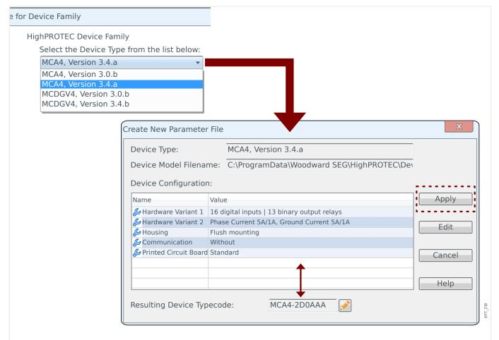
Fig. 4: For offline creation of a configuration file, you are first asked for the device name and version. After this, specify the particular device variant.
