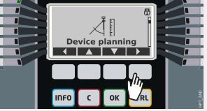
This setting can be found in the Device planning menu branch (which can be seen, for example, in the Reference Manual). The purpose of the parameter is to activate (or deactivate) the protection function »I[2]« (i. e. the 2<sup>nd</sup> stage of the Overcurrent protection).
