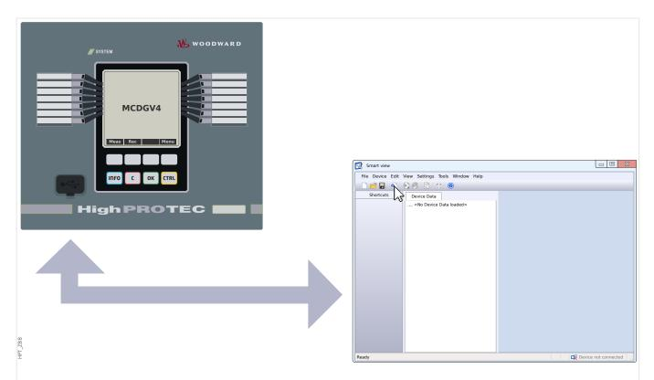
Fig. 1: Connect the PC to the protection device and within Smart view, specify the connection settings.
