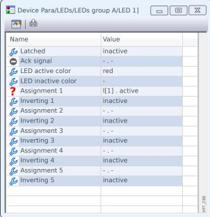
The **question mark** token, either in the heading of the display or as a bold red sign within the *Smart view* dialog, indicates that a validity or consistency problem has been detected.
