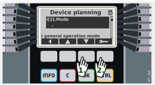
Then press the "▼" (Down) Softkey repeatedly, until the required setting can be seen in the display.
