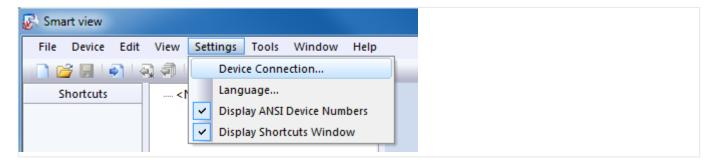
• Select "Serial Connection" in the dialog. Then you can pick the particular COM port to which the protective device is connected from the selection list.
