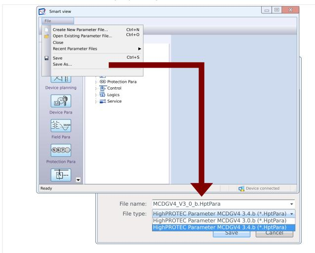
Fig. 6: Converting a configuration file for the MCDGV4 from version "3.0.b" to "3.4.b".
