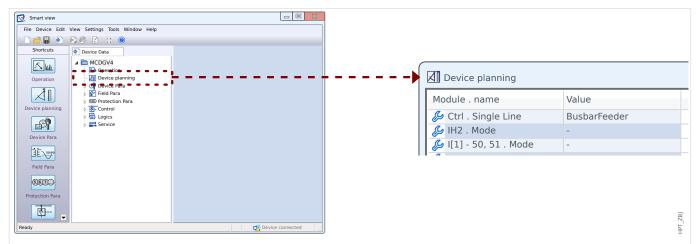
Fig. 8: Double click [Device planning] and select the required protection and supervision modules.
