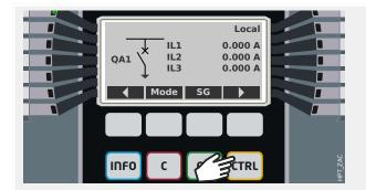
By pressing the »CTRL« key you enter a screen showing the single line, and you have direct access to related control functions.
