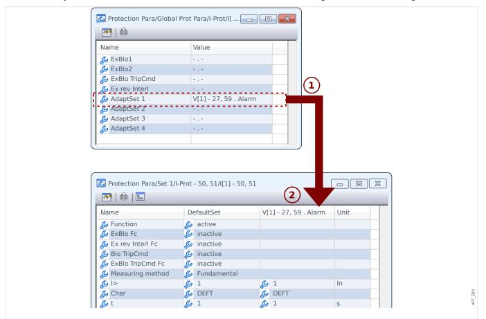
Fig. 3: An assignment to an Adaptive Set parameter adds alternative values to Setting Group parameters.
