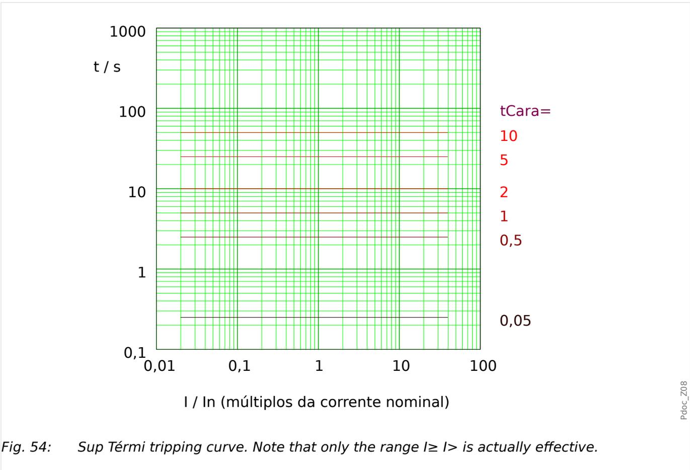
Fig. 54: Sup Térm tripping curve. Note that only the range  $I \geq I >$  is actually effective.
