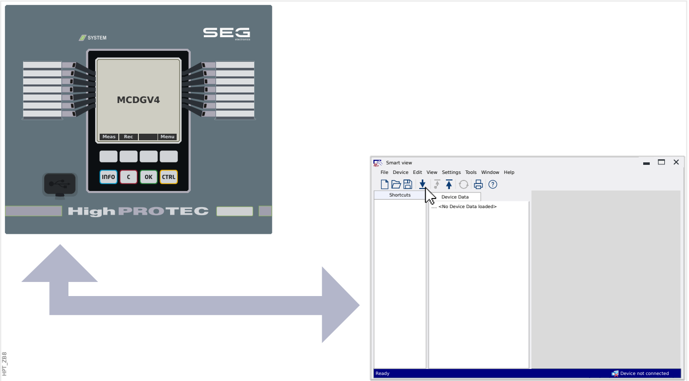
Fig. 1: Connect the PC to the protection device and within Smart view, specify the connection settings.
