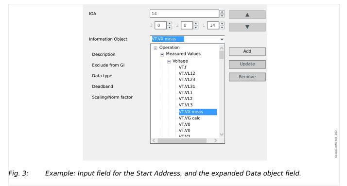
After the data object has been selected, some more input fields become visible, depending on the type of data object and depending on the selected SCADA protocol.
