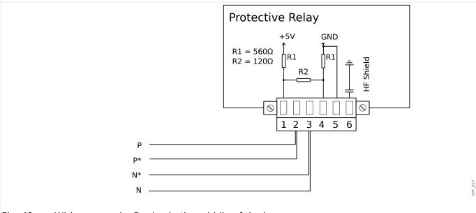
Fig. 49: Wiring example, Device in the middle of the bus
