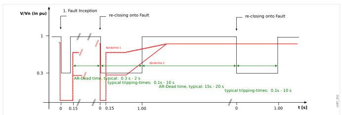
Fig. 148: Run of voltage curve during an unsuccessful two-shot auto reclosure; source: VDE-AR-N 4110/4120.
