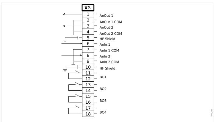
Fig. 30: Terminal Marking.
