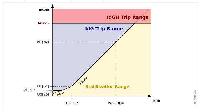
Fig. 91: Pickup value »IdG>>« of the earth differential current based on the rated current »Ib« of the related protection object.
