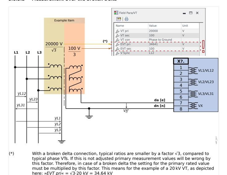
After the voltage inputs have been connected correctly the residual voltage is measured with the following setting:
