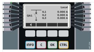
Fig. 159: Control Page Example, with the "Circuit Breaker" in intermediate position.
