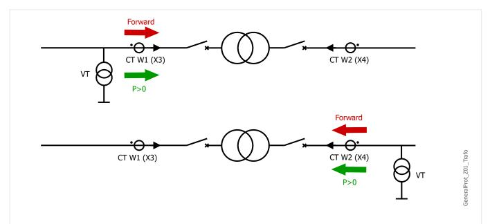
Fig. 72: Direction definitions of current and power for the MCDTV4.
