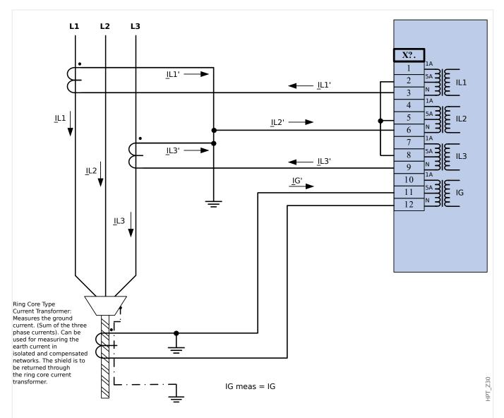
Fig. 25: Two phase current measurement (Open Delta); In secondary = 5 A. Earth-current measuring via cable-type current transformer; IGnom secondary = 5 A.
