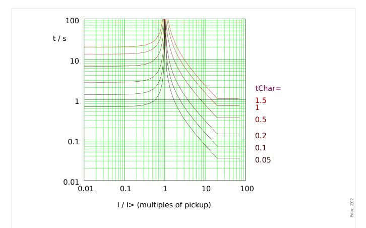
Fig. 93: VINV: reset delay (left half,  $I < I_>$ ) and trip delay (right half,  $I > I_>$ ), example for  $I_{max} = 20 \cdot I_>$ .
