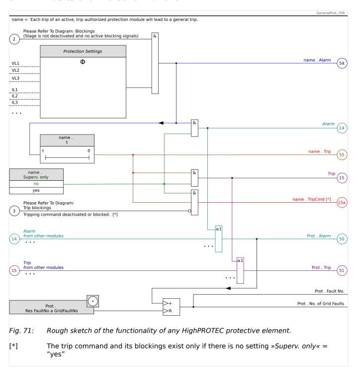
This diagram shows the basic idea behind a protective element. (Nevertheless, keep in mind that device-specific or protection-specific deviations are possible: Some devices do not feature voltage measurement, other do not feature current measurement, for some protection elements other timers and/or phase-specific algorithms are required, etc. So, for the exact functionality of a protection module please consult the respective chapter.)
