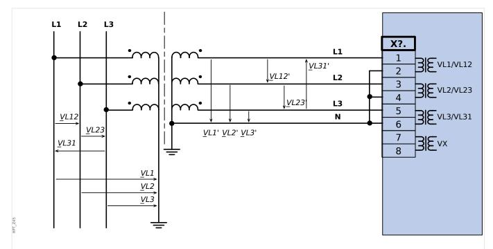
Fig. 35: VT Wye: Three-phase voltage measurement - wiring of the measurement inputs: "star-connection"
