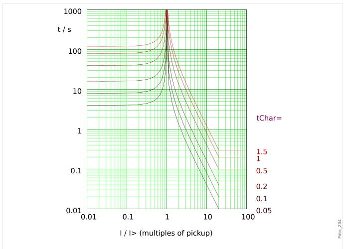
Fig. 94: EINV: reset delay (left half,  $I < I_>$ ) and trip delay (right half,  $I > I_>$ ), example for  $I_{max} = 20 \cdot I_>$ .
