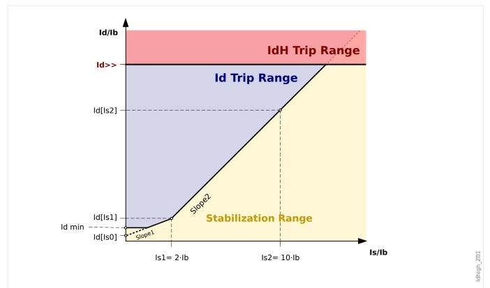
Fig. 88: Unrestrained High-set Differential Protection Step IdH.
