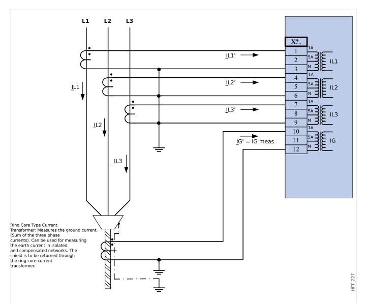
Fig. 22: Three phase current measurement; In secondary = 1 A. Earth-current measuring via cable-type current transformer; IGnom secondary = 1 A.
