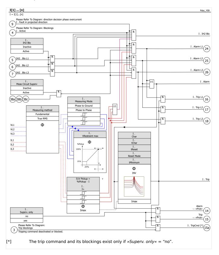
Remark: For the sake of simplicity, the diagram above does not show the fact that in case of [Field Para / VT] >VT con« = "Phase to Phase", the parameter >I[x]«. Measuring Mode is internally re-set to "Phase to Phase", independent of its configured value (see the Notice in  $\hookrightarrow$ Chapter 5.8.3).
