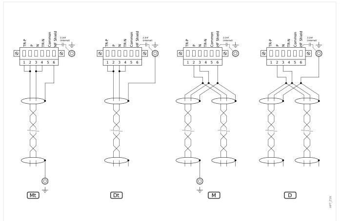
Fig. 51: Shielding Options (2-wire + Shield)
