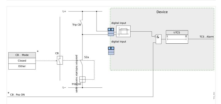
Connection example: Trip circuit supervision with only one CB auxiliary contact »Aux Fig. 156: ON« (52a).
