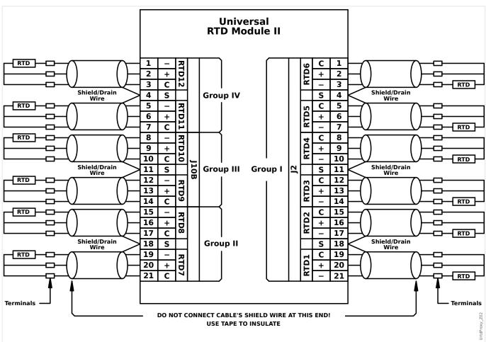
See the figure above for wiring of RTDs to the URTD inputs. Use three-conductor shielded cable. Note the connection rules in the figure. When making connections to a two-lead RTD, connect two of the cable conductors to one of the RTD leads as shown. Make this
