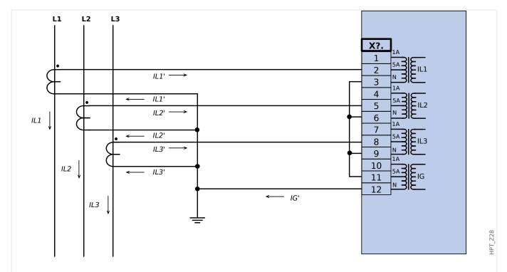
Fig. 23: Three phase current measurement; In secondary = 5 A. Earth-current measuring via Holmgreen-connection; IGnom secondary = 5 A.
