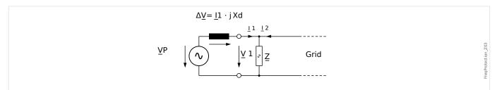
Fig. 128: Equivalent circuit at synchronous generator in parallel with the mains.
