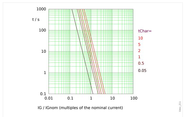
Fig. 116: I4T tripping curve, example diagram for measured (non-sensitive) earth/ground current (51G). Note that only the range  $IG > I_{G>}$  is actually effective.
