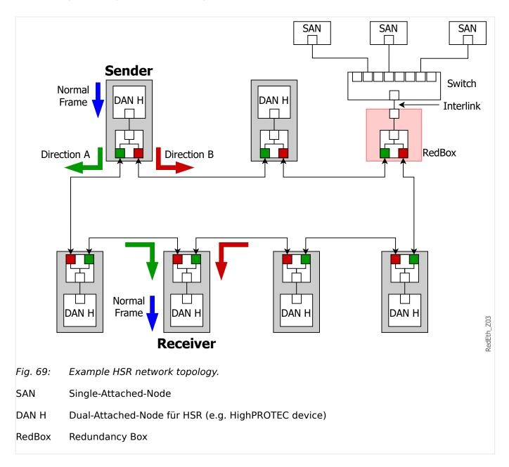
Every node in the ring must be HSR-capable. In cases where a non-HSR-capable device needs to communicate with one or more nodes in the ring, an HSR-RedBox (Redundancy Box) must be used.
