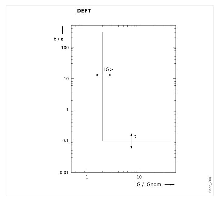
Trip delay for  $IG > I_{G>}$ , settable via [Protection Para / Set 1...4 / I-Prot / IG[x]] »t«.
