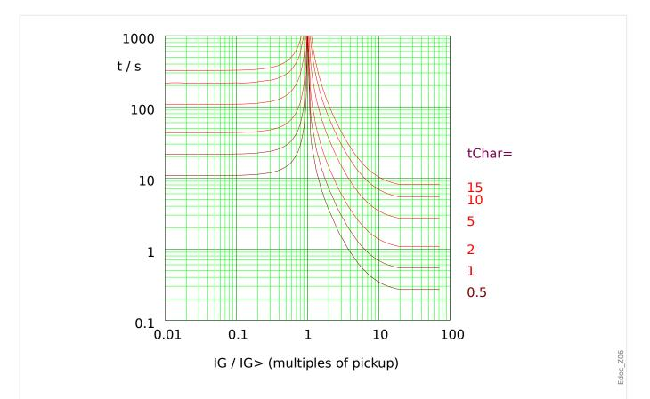
Fig. 110: VINV: reset delay (left half,  $IG < I_{G>}$ ) and trip delay (right half,  $IG > I_{G>}$ ), example for  $I_{max} = 20 \cdot I_{G>}$ .
