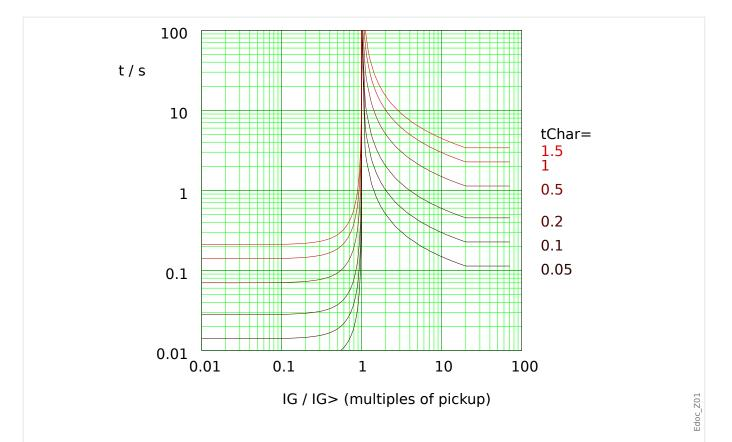
Fig. 104: NINV: reset delay (left half,  $IG < I_{G>}$ ) and trip delay (right half,  $IG > I_{G>}$ ), example for  $I_{max} = 20 \cdot I_{G>}$ .
