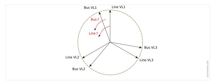
If the generator frequency fBus is not equal to the mains frequency fLine, it results in a slip frequency  $\Delta F = |\text{fBus -fLine}|$  between the two system frequencies.
