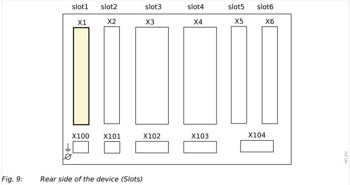
The type of power supply card and the number of digital inputs on it used in this slot is dependent on the ordered device type. The different variants have a different scope of functions.
