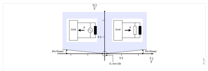
Fig. 140: Method 1: Power Angle Supervision.
