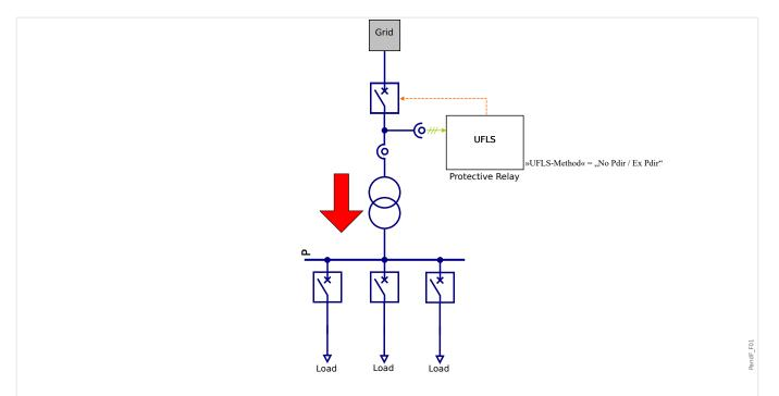
Fig. 143: Grid without or low decentalized infeed, directional dependency is not required (classic load shedding).
