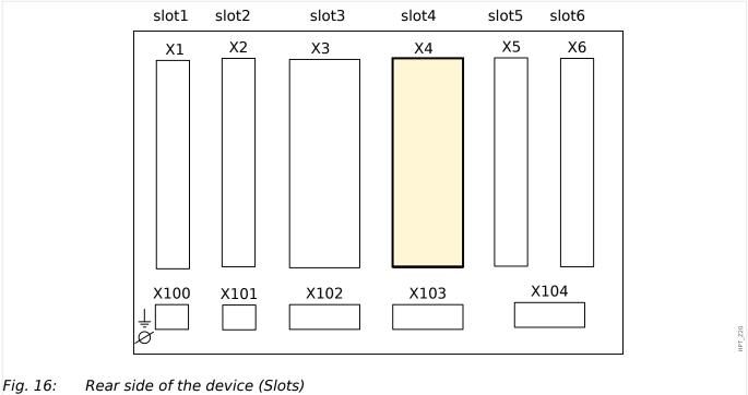
This slot contains the current transformer measuring inputs for the W2 side.
