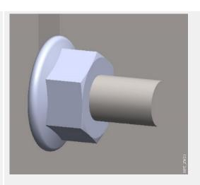
Screw hexagon nuts (4 x 1-364-88) to the side plates (recommended torque: 2.4Nm)
