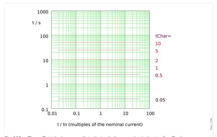
Fig. 100: Therm Flat tripping curve. Note that only the range  $I > I_{>}$  is actually effective.
