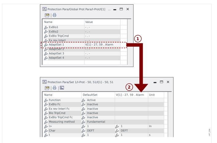
Fig. 2: An assignment to an Adaptive Set parameter adds alternative values to Setting Group parameters.
