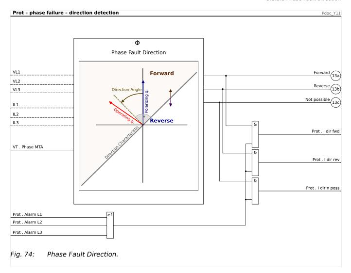
The MCDTV4 evaluates the angle between the current of the phase with the highest current (*Operating quantity*) and the phase-to-phase voltage of the other phases (Polarizing quantity). For three-phase-faults where the phase-to-phase-voltage is too low a voltage memory is used.
