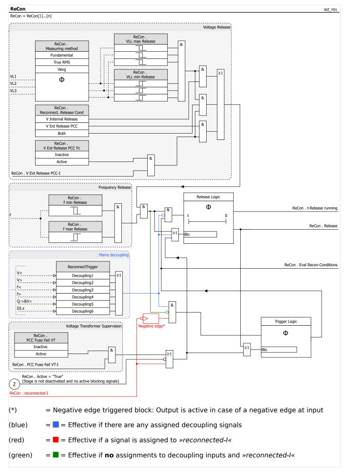
Generally, the function can be divided into a trigger-logic and a release-logic. The trigger part defines when the function starts with the evaluation of the reconnection conditions. The evaluation phase including the mains settle timer »t-Release Blo« is defined from the release logic.
