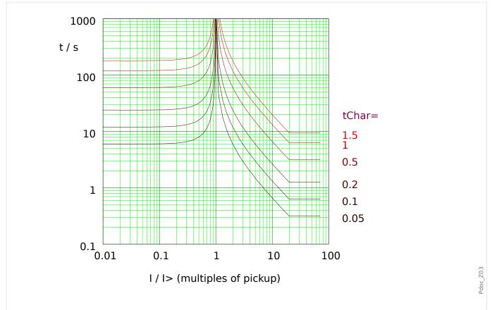
Fig. 95: LINV: reset delay (left half,  $I < I_>$ ) and trip delay (right half,  $I > I_>$ ), example for  $I_{max} = 20 \cdot I_>$ .
