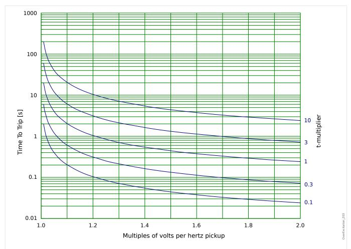
Fig. 122: Characteristic / Curve Shape: INV C
