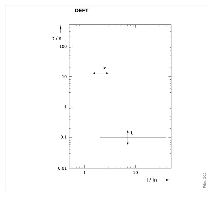
Trip delay for  $I > I_>$ , settable via [Protection Para / Set 1...4 / I-Prot / I[x]] »t«.
