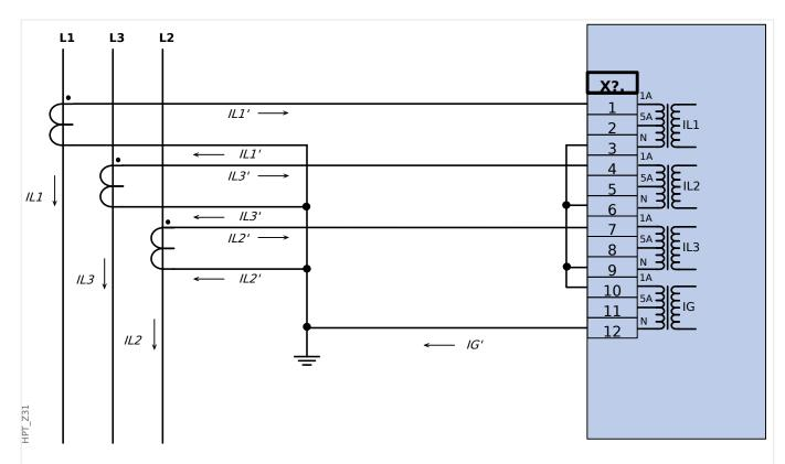
Fig. 26: Three phase current measurement; In secondary = 1 A. Earth-current measuring via Holmgreen-connection; IGnom secondary = 1 A.
