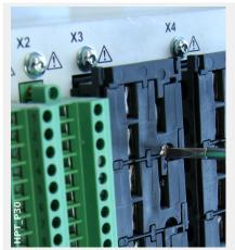
For either connection type, the first step is to remove the terminals from the device by opening the screws.
