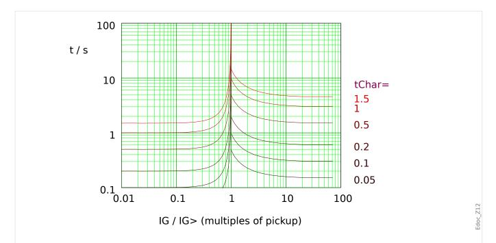
Fig. 108: RINV: reset delay (left half,  $IG < I_{G>}$ ) and trip delay (right half,  $IG > I_{G>}$ ), example for  $I_{max} = 20 \cdot I_{G>}$ .
