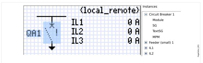
Fig. 158: Control Page Example, with the "Circuit Breaker" being highlighted.
