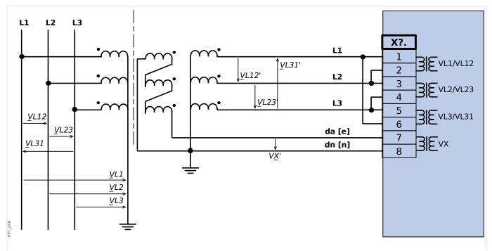
Fig. 38: Three-phase voltage measurement - wiring of the measurement inputs: "delta-connection"Measurement of the residual voltage VG via auxilliary windings (e-n) "broken delta"
