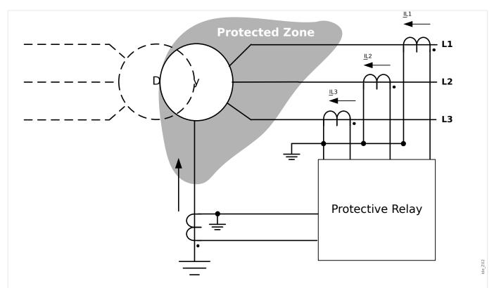
Fig. 89: Protection principle of Ground Current Differential Protection connected on wye-side winding of a transformer.
