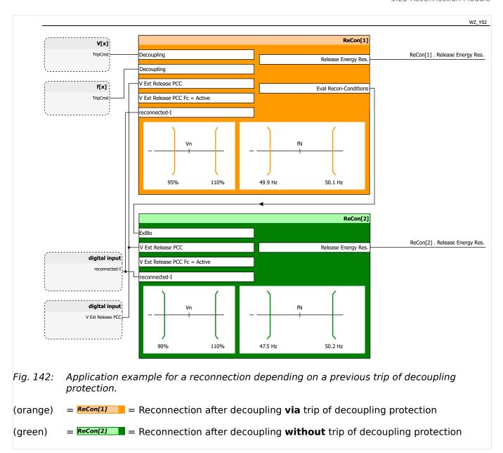
The release ranges (orange) that are used after a trip of decoupling protection are smaller than the release ranges (green) without a previous trip. The example above configures the first reconnection instance, »ReCon[1]«, for the small (orange) ranges, and the decoupling functions are assigned to this instance.
