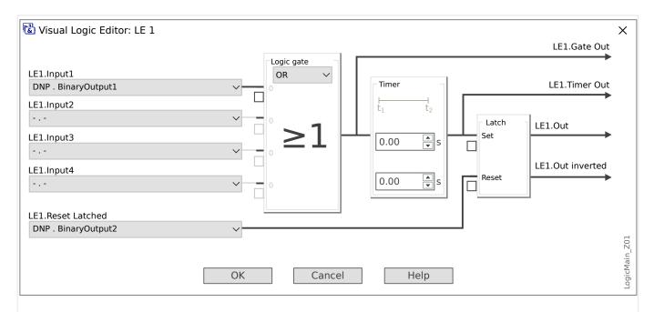
Fig. 65: Setting example from Smart view, to make a steady state signal from a DNP output signal.
