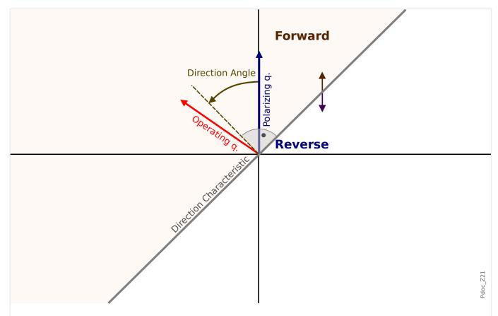
Fig. 73: Principle of Phase Fault Direction Detection.
