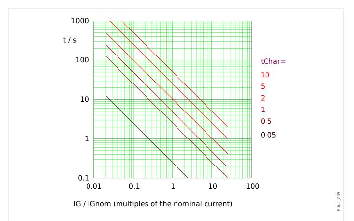
Fig. 114: IT tripping curve, example diagram for measured (non-sensitive) earth/ground current (51G). Note that only the range  $IG > I_{G>}$  is actually effective.
