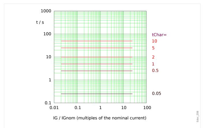
Fig. 113: Therm Flat tripping curve, example diagram for measured (non-sensitive) earth/ground current (51G). Note that only the range  $IG > I_{G>}$  is actually effective.
