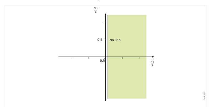
Fig. 146: Method 2 (Pure Active Power Supervision): »UFLS-Method« = "Pure Active Power Superv".
