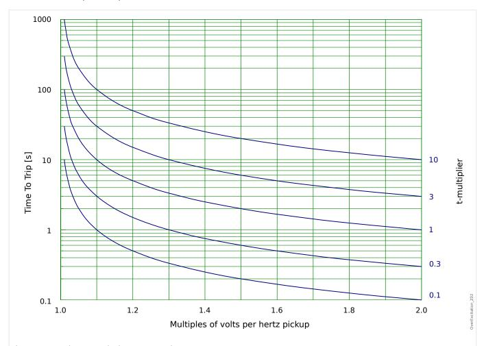
Fig. 121: Characteristic / Curve Shape: INV B
