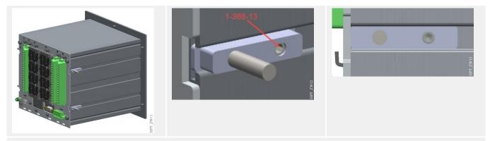
Position all four slot nuts (1-346-97) flush with the back of the HighPROTEC and secure with grub screws (1-388-13)(recommended torque: 1.5Nm). Caution: Use original grub screws (1-388-13) with Tuflok coating. Otherwise safety cannot be guaranteed.
