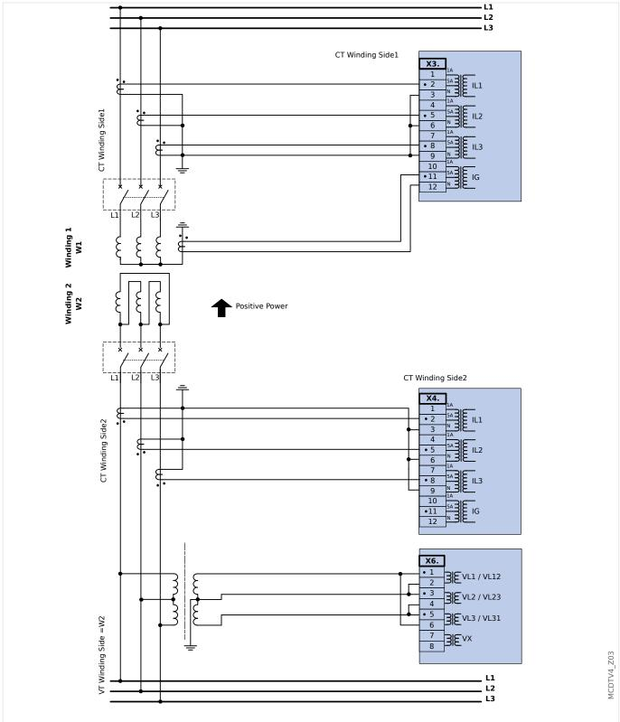
Fig. 41: DY Transformer with Phase Differential Protection, REF on W1 and VT on W2 (V-Connection).
