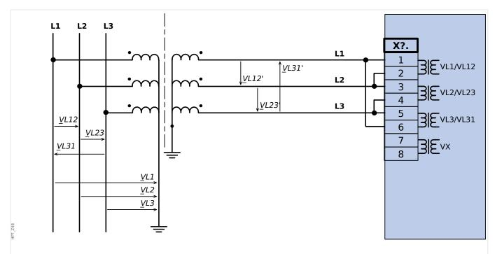
Fig. 37: Three-phase voltage measurement - wiring of the measurement inputs: "delta-connection"
