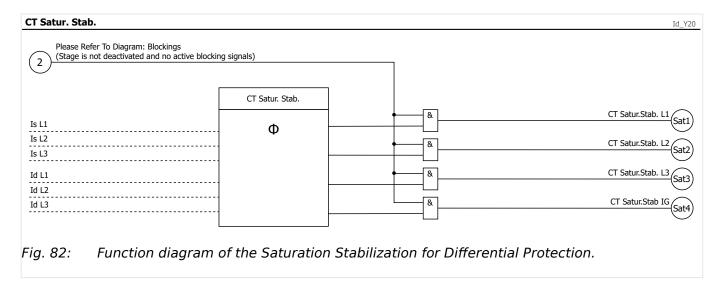
The stabilization is triggered as soon as an external fault is detected, which is evaluated continuously. The differential protection is robust against CT saturation as long as the external fault and therefore the stabilization continues. The stabilization is stopped if an internal fault is detected.
