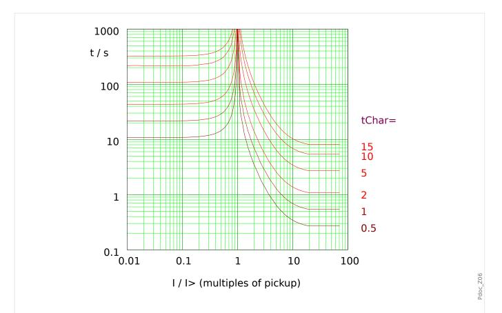
Fig. 98: VINV: reset delay (left half,  $I < I_>$ ) and trip delay (right half,  $I > I_>$ ), example for  $I_{max} = 20 \cdot I_>$ .
