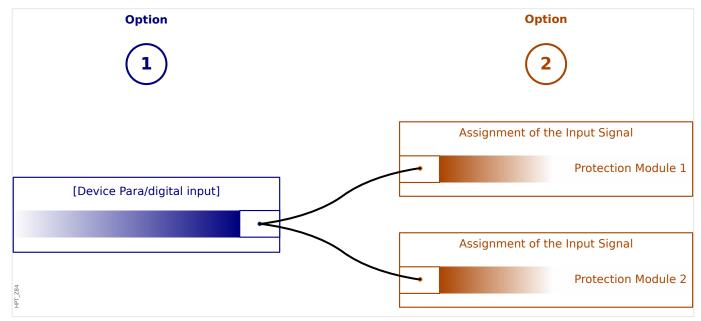
**Option 1:** Assigning a Digital Input onto one or mutliple modules.
