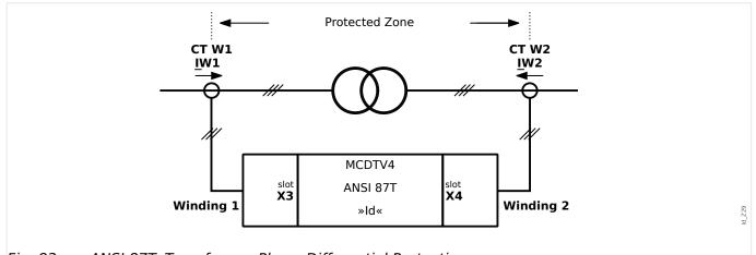
Fig. 83: ANSI 87T: Transformer Phase Differential Protection.
