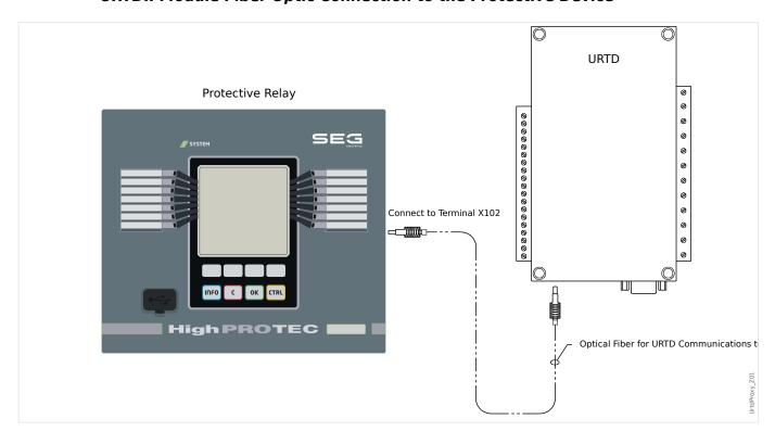
The figure above shows the fiber optic connections between the URTDII Module and the protective device. The protective device supports the optical fiber connection.
