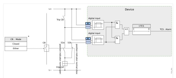
Fig. 155: Connection example: Trip circuit supervision with two CB auxiliary contacts »Aux ON« (52a) and »Aux OFF« (52b).
