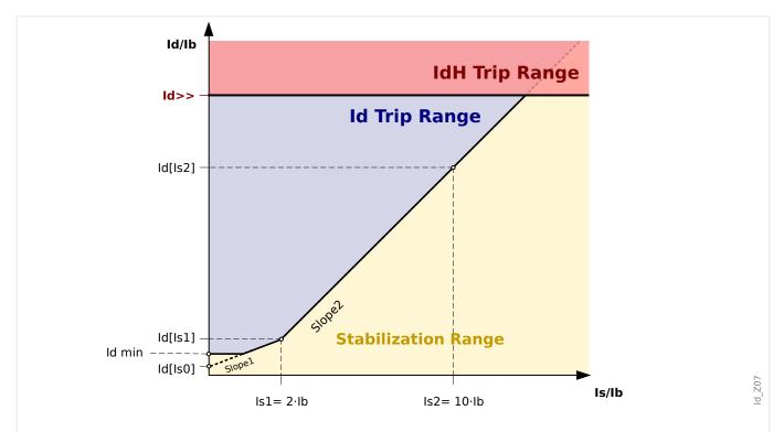
Fig. 86: Tripping curves of the »Id« (blue area) and of the »IdH« (red area) protection functions.
