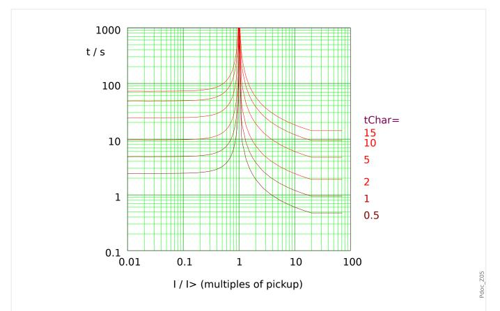
Fig. 97: MINV: reset delay (left half,  $I < I_>$ ) and trip delay (right half,  $I > I_>$ ), example for  $I_{max} = 20 \cdot I_>$ .
