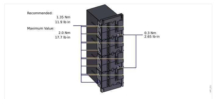
Fig. 179: Plug-in Connector with Integrated Short-Circuiter (Conventional Current Inputs)
