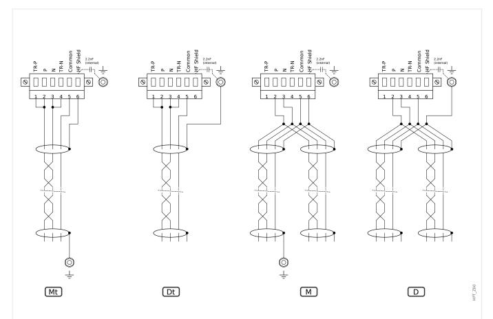
Fig. 52: Shielding Options (3-wire + Shield)
