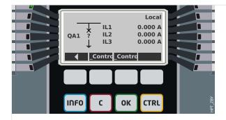
Fig. 162: Control Page Example, with the "Circuit Breaker" in faulty (or implausible) position.
