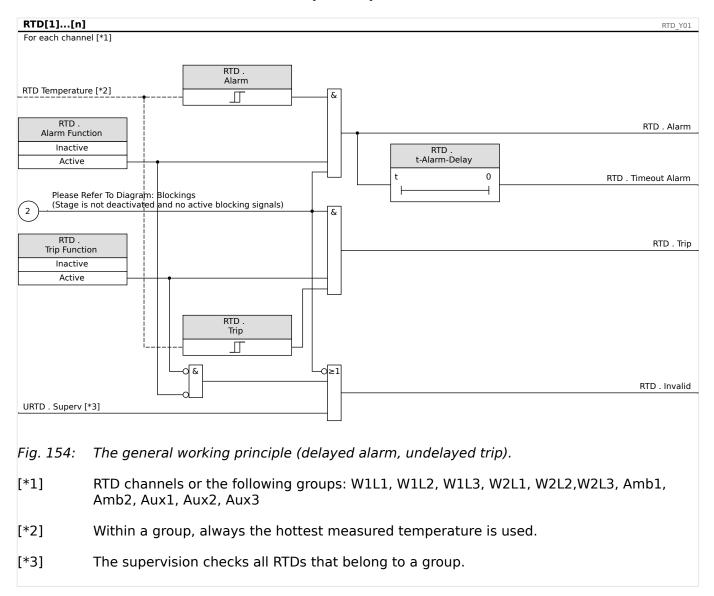
The diagram shows the general working principle (delayed alarm, undelayed trip) of each of the RTD sensors. Note that some text-labels had to be simplified, to make the diagram valid for each group. Please consult the Reference Manual for exact listings of available parameters and signals.
