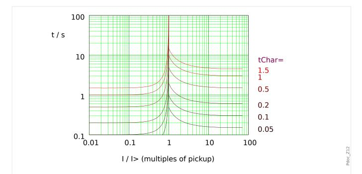
Fig. 96: RINV: reset delay (left half,  $I < I_>$ ) and trip delay (right half,  $I > I_>$ ), example for  $I_{max} = 20 \cdot I_>$ .
