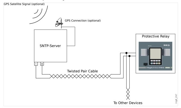
The location of the IRIG-B interface depends to the device type. Please refer to the wiring diagram supplied with the protective device.
