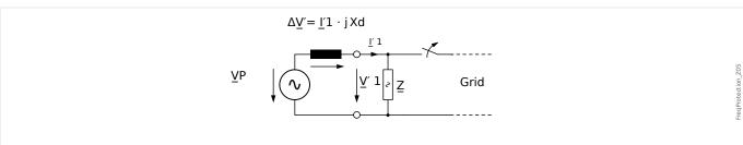
Fig. 130: Equivalent circuit at mains failure.
