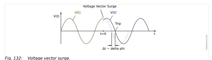
As shown in the voltage/time diagram the instantaneous value of the voltage jumps to another value and the phase position changes. This is called phase or vector surge.
