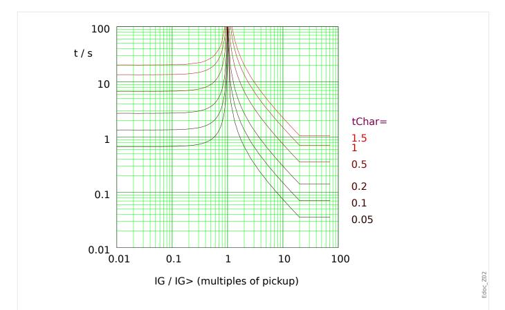
Fig. 105: VINV: reset delay (left half,  $IG < I_{G>}$ ) and trip delay (right half,  $IG > I_{G>}$ ), example for  $I_{max} = 20 \cdot I_{G>}$ .
