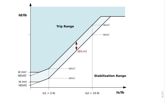
Fig. 87: Temporary Dynamic Raise of the Static Tripping Characteristic.
