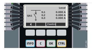
Fig. 161: Control Page Example, with the "Circuit Breaker" in open position.
