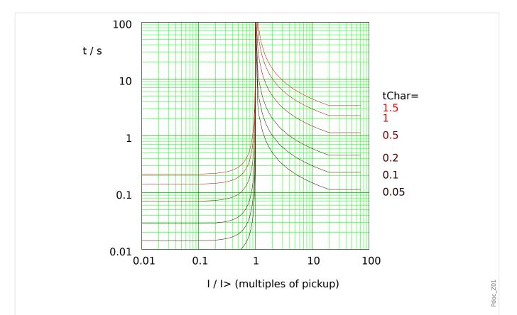
Fig. 92: NINV: reset delay (left half,  $I < I_>$ ) and trip delay (right half,  $I > I_>$ ), example for  $I_{max} = 20 \cdot I_>$ .
