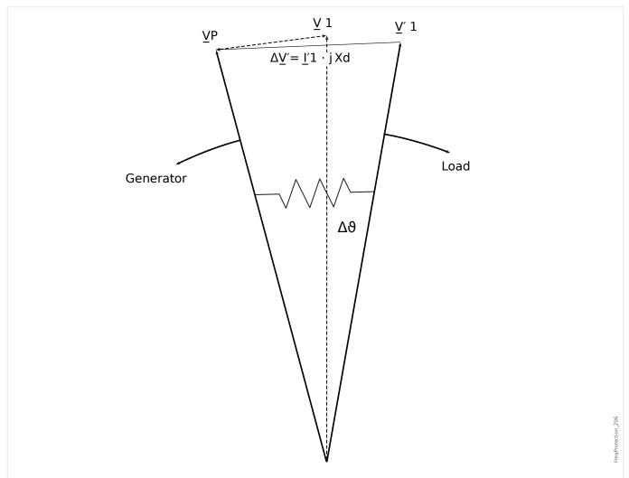
Fig. 131: Voltage vectors at mains failure.
