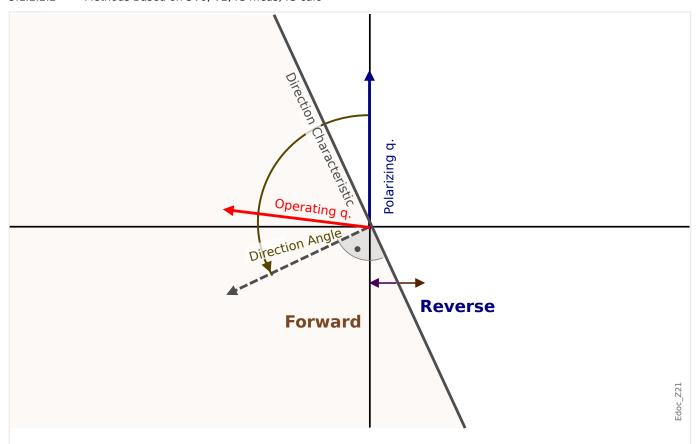
Fig. 75: Principle of direction determination for all methods except " $cos(\phi)$ ", " $sin(\phi)$ ".
