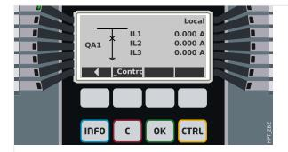
Fig. 160: Control Page Example, with the "Circuit Breaker" in closed position.
