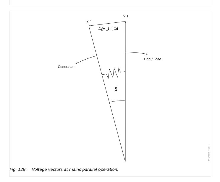
The rotor displacement angle between stator and rotor is dependent on the mechanical moving torque of the generator. The mechanical shaft power is balanced with the electrical fed mains power and, therefore the synchronous speed keeps constant.
