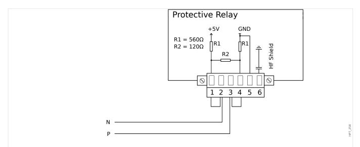
Fig. 50: Wiring example, Device at the end of the bus. (Setting wire jumpers to activate the integrated Terminal Resistor.)
