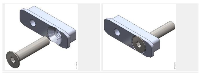
Countersunk screw (1-388-12) into slot nut (1-346-97) (recommended torque: 1.1Nm)
