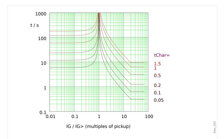
Fig. 107: LINV: reset delay (left half,  $IG < I_{G>}$ ) and trip delay (right half,  $IG > I_{G>}$ ), example for  $I_{max} = 20 \cdot I_{G>}$ .
