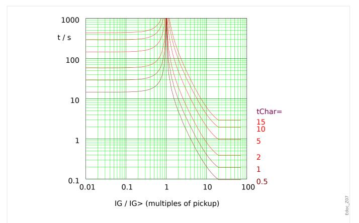
Fig. 111: EINV: reset delay (left half,  $IG < I_{G>}$ ) and trip delay (right half,  $IG > I_{G>}$ ), example for  $I_{max} = 20 \cdot I_{G>}$ .
