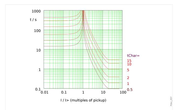
Fig. 99: EINV: reset delay (left half,  $I < I_>$ ) and trip delay (right half,  $I > I_>$ ), example for  $I_{max} = 20 \cdot I_>$ .
