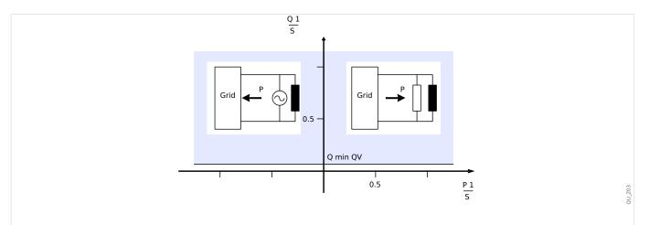
Fig. 141: Method 2: Pure Reactive Power Supervision.
