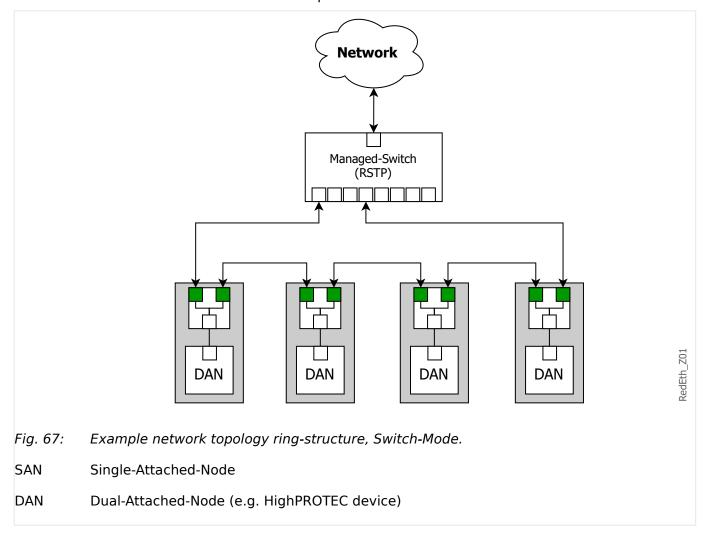
In a closed ring, the managed switch automatically blocks one of the two paths. In case of a failure or disruption, the managed switch then utilizes the remaining functional path.
