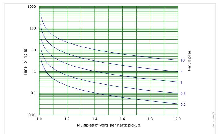
Fig. 120: Characteristic / Curve Shape: INV A
