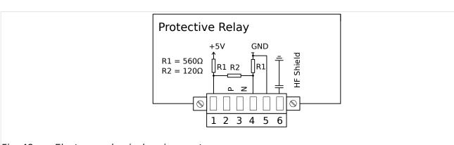
Fig. 48: Electro-mechanical assignment
