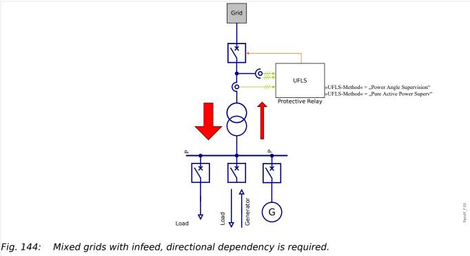
The power flow direction detection (if activated) will block the shedding of sub-grids in case of an under frequency situation of those sub-grids that stabilize the frequency. The sub-grid will be shed only if it decreases the frequency (by consuming active power).
