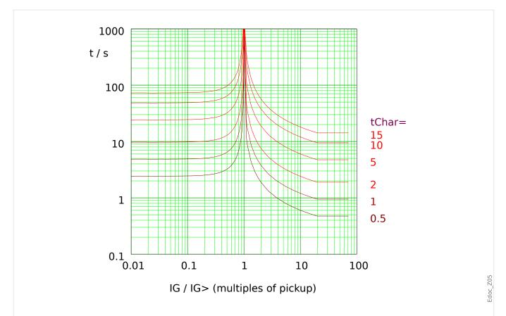
Fig. 109: MINV: reset delay (left half,  $IG < I_{G>}$ ) and trip delay (right half,  $IG > I_{G>}$ ), example for  $I_{max} = 20 \cdot I_{G>}$ .
