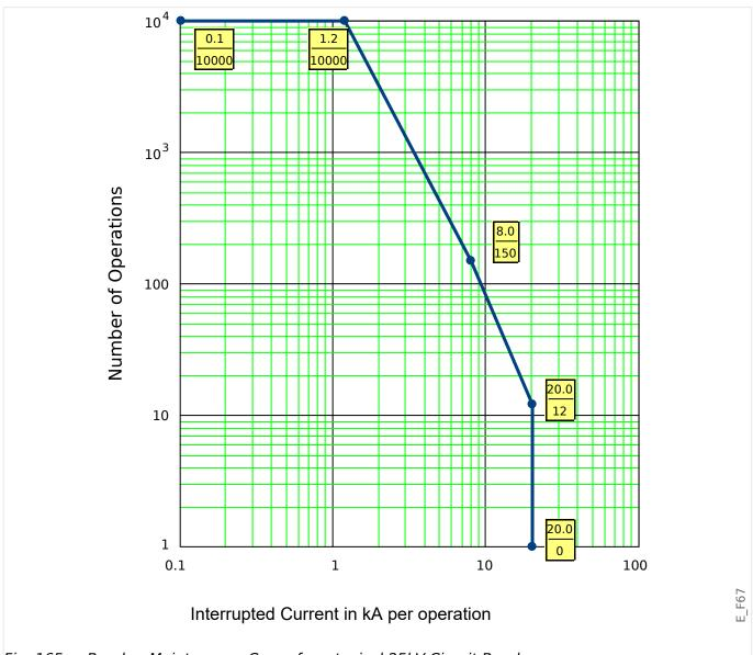
Fig. 165: Breaker Maintenance Curve for a typical 25kV Circuit Breaker
