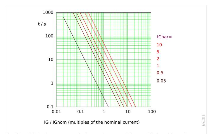
Fig. 115: I2T tripping curve, example diagram for measured (non-sensitive) earth/ground current (51G). Note that only the range  $IG > I_{G}$  is actually effective.
