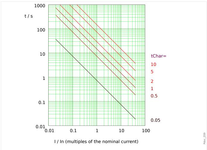
Fig. 101: IT tripping curve. Note that only the range  $I > I_{>}$  is actually effective.
