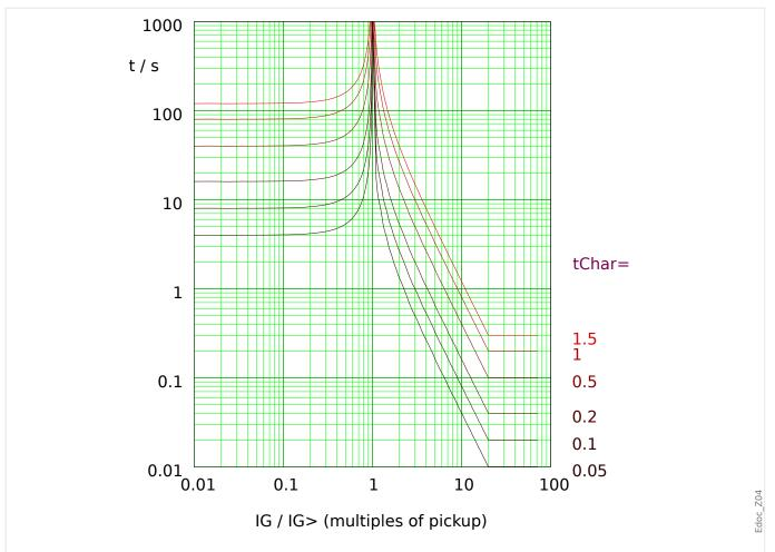
Fig. 106: EINV: reset delay (left half,  $IG < I_{G>}$ ) and trip delay (right half,  $IG > I_{G>}$ ), example for  $I_{max} = 20 \cdot I_{G>}$ .
