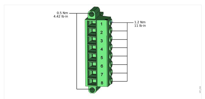
Fig. 180: Voltage measurement terminals of measuring card "TU" ( $\hookrightarrow 3.8.1 \text{ TU}$  - Voltage Measuring Inputs).
