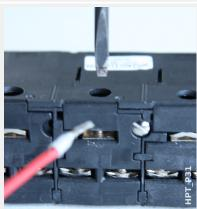
For the pin-terminal connection type, insert the cables and fasten them by the screws that are located at the side of the input card.
