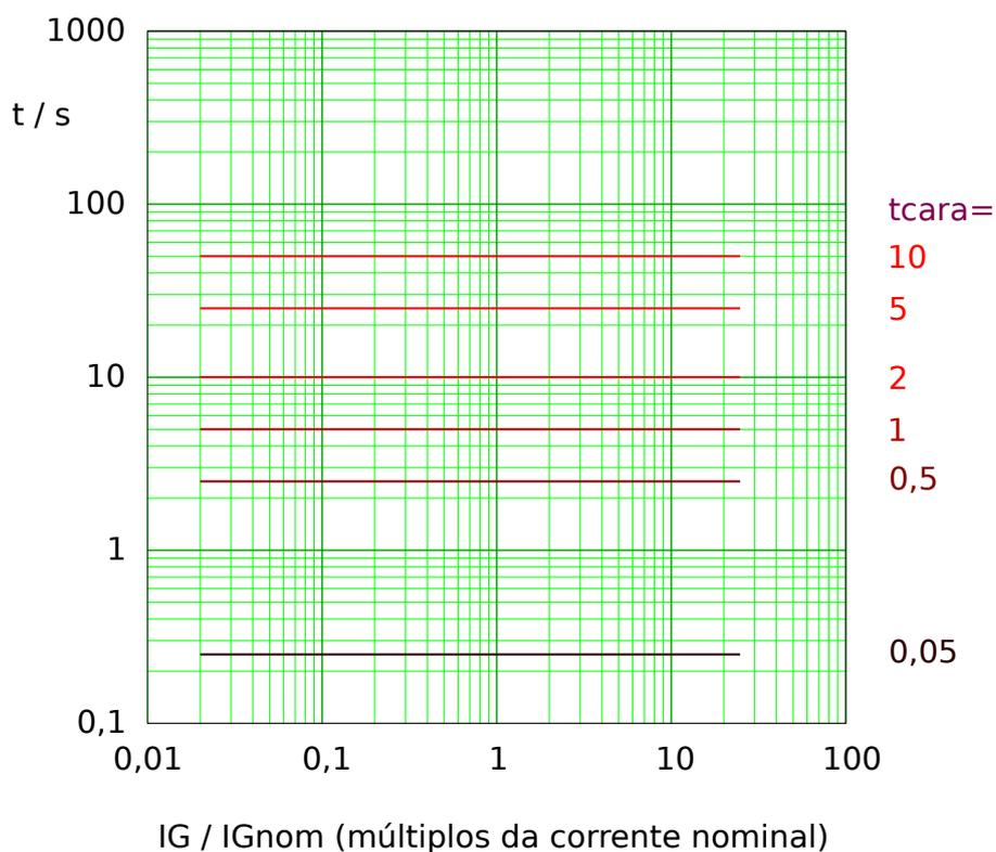
Fig. 85: Sup Térmi tripping curve. Note that only the range  $IG \geq IG>$  is actually effective.
