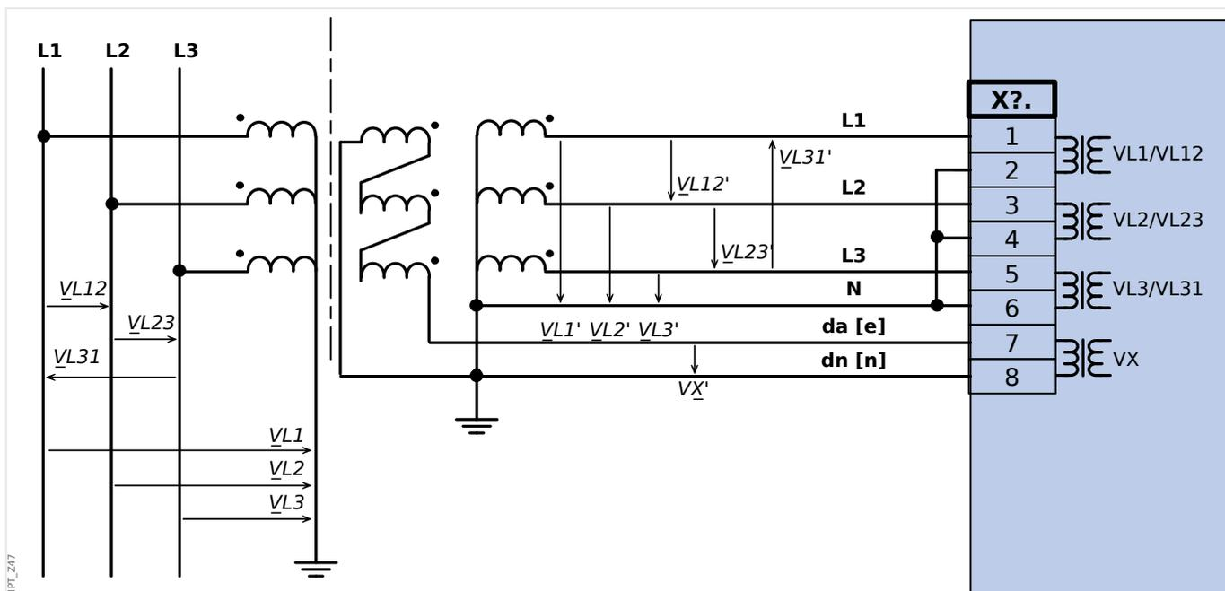
Fig. 35: VT Wye com conexão Broken Delt.
