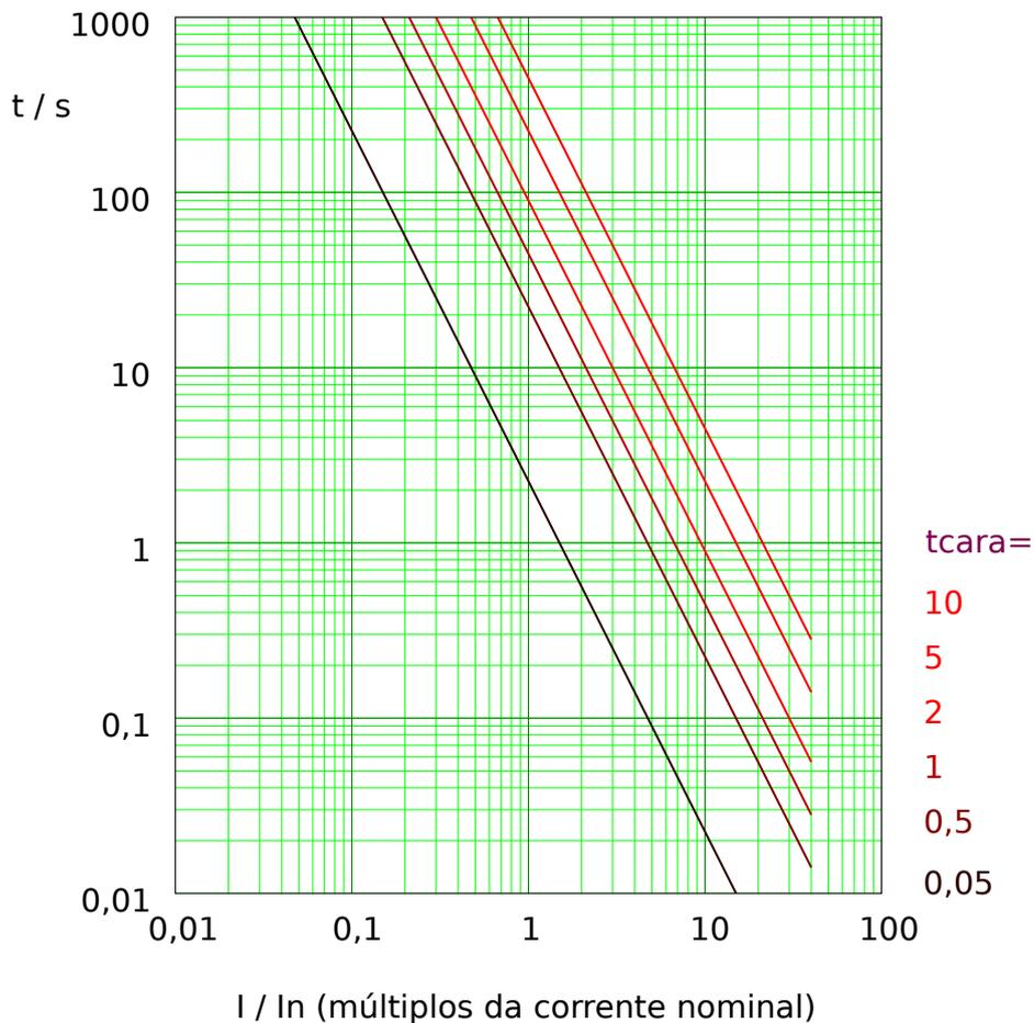
Fig. 83: I2T tripping curve. Note that only the range  $I \geq I_n$  is actually effective.
