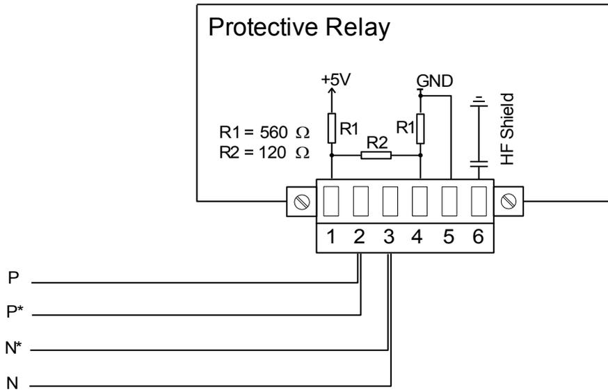
Wiring example, Device **at the end** of the bus
