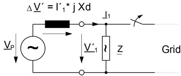
In case of mains failure or auto reclosing the generator suddenly feeds a very high consumer load. The rotor displacement angle is decreased repeatedly and the voltage vector  $V_1$  changes its direction ( $V'_1$ ).
