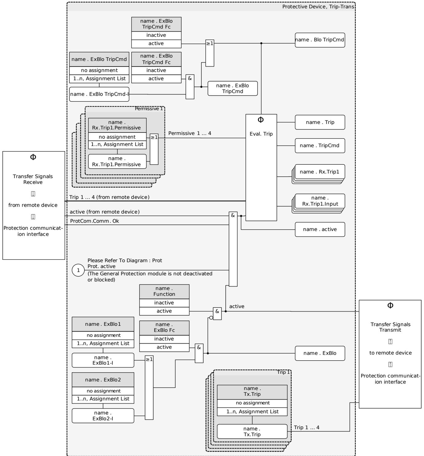
Functionality of the Trip-Trans module. The sub-routine "Eval. Trip" is detailed in the following diagram.
