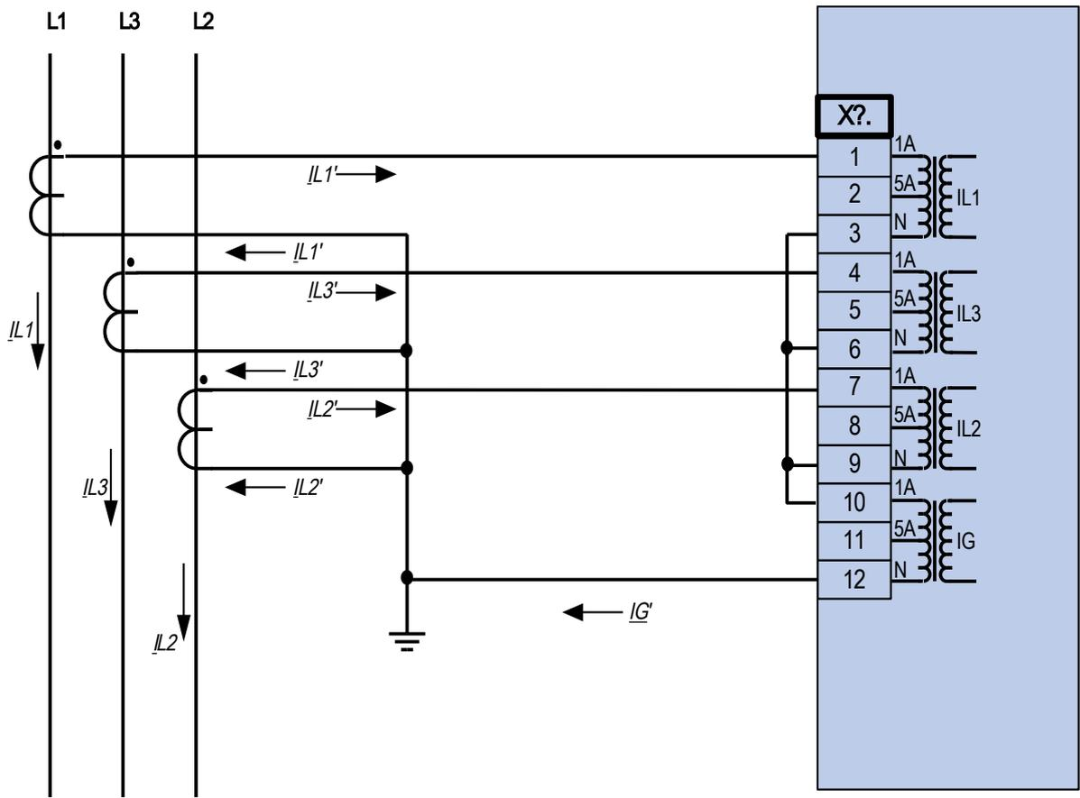
Three phase current measurement;  $I_n$  secondary = 1 A.
