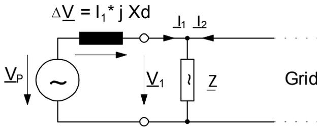
Voltage vectors at mains parallel operation.
