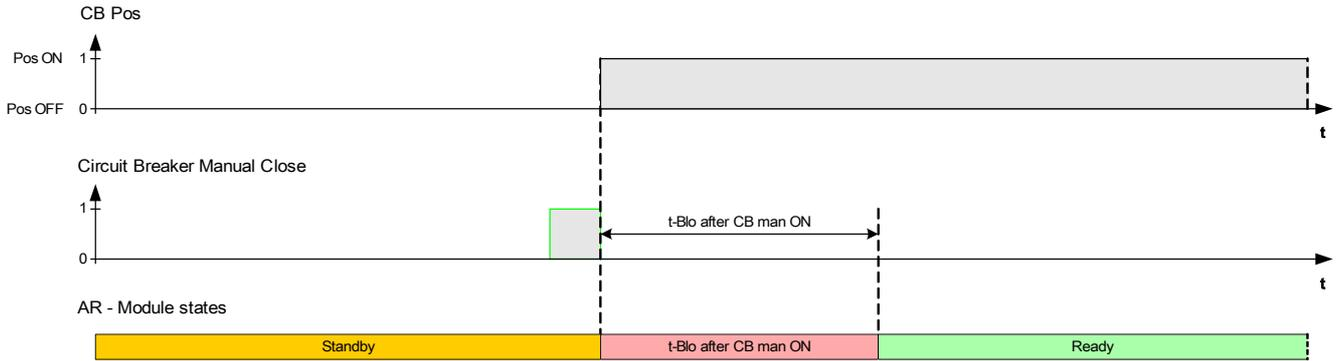
*Protection Trip while Manual Close Blocking time is Timing*
