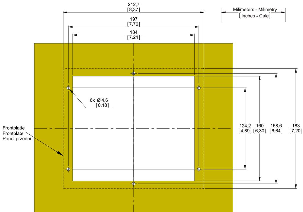
B2 Housing Door Cut-out (8-Pushbutton Version). (All dimensions in mm, except dimensions in brackets [inch].)
