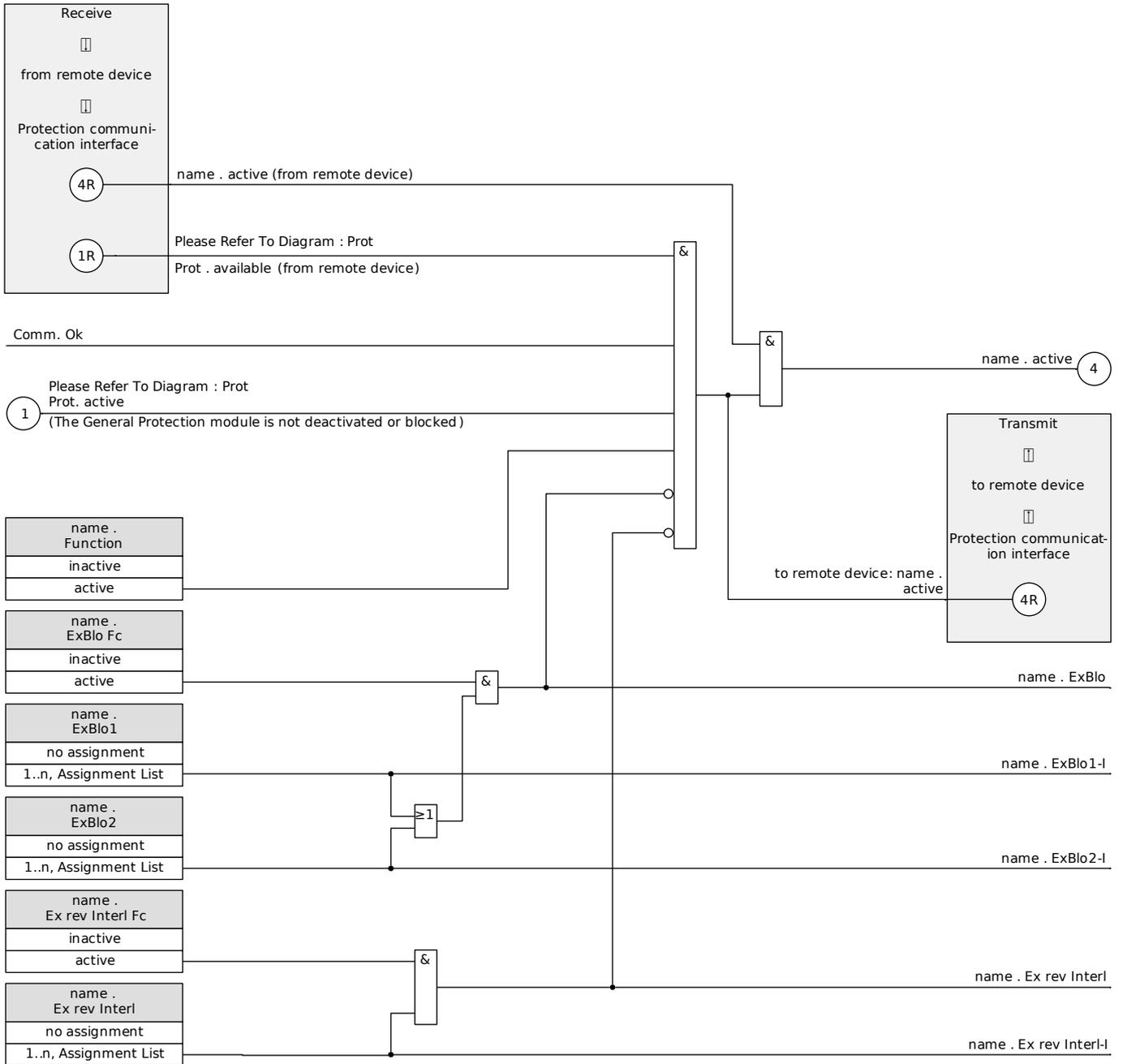
The following diagram is applies to the Q->&V< Protection:
