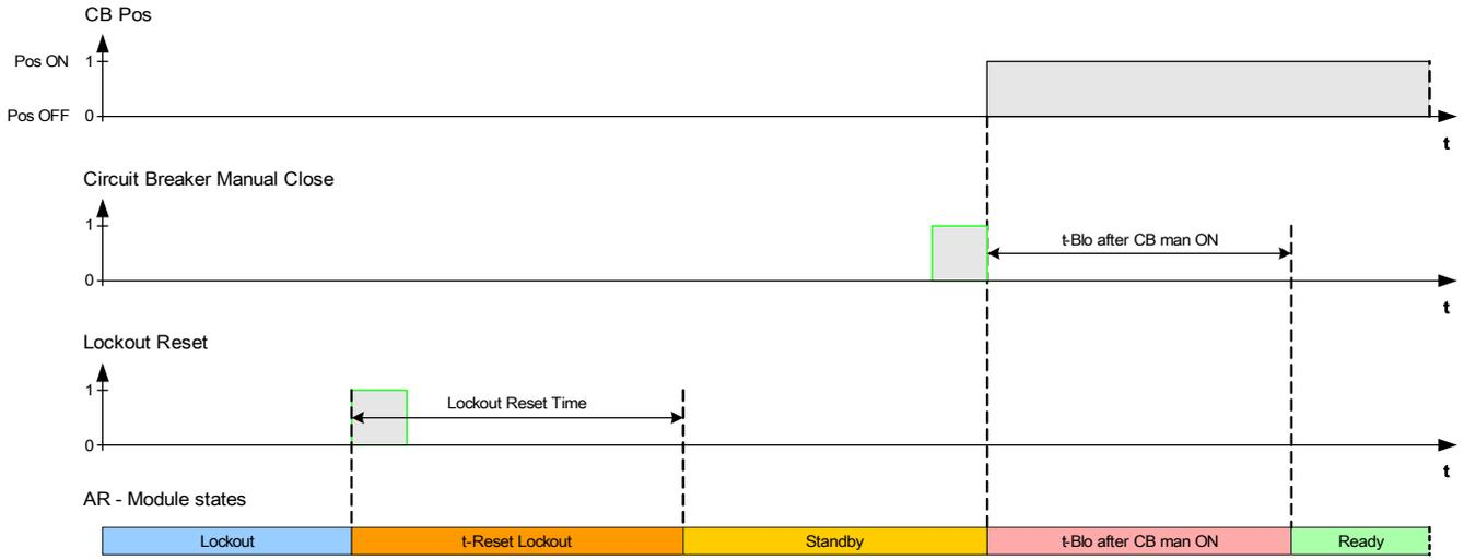
*AR Lockout Reset Logic in case lockout Reset coming after manual breaker closed*
