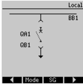
The truck of a withdrawable circuit breaker has to be managed as an individual switchgear. There is no fixed connection between the circuit breaker and the truck. An interlocking has to be set by the User because it is not allowed to withdraw the breaker as long as it is in the closed position. The circuit breaker can be switched in the withdrawn and in the non-withdrawn position.
