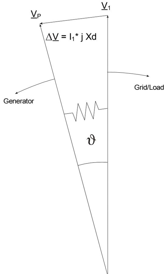
The rotor displacement angle between stator and rotor is dependent on the mechanical moving torque of the generator. The mechanical shaft power is balanced with the electrical fed mains power and, therefore the synchronous speed keeps constant.
