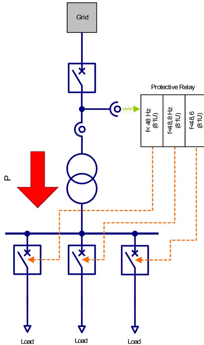
Centralized Under Frequency Load Shedding within grids with temporary power supply.
