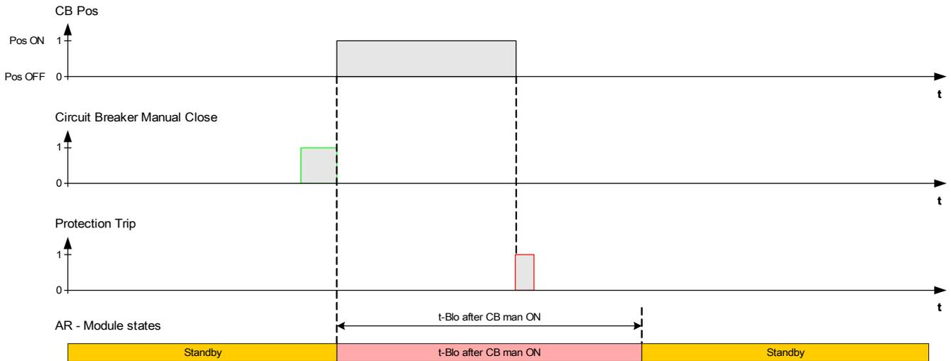
*AR Lockout Reset Logic in case lockout Reset coming before manual breaker closed*
