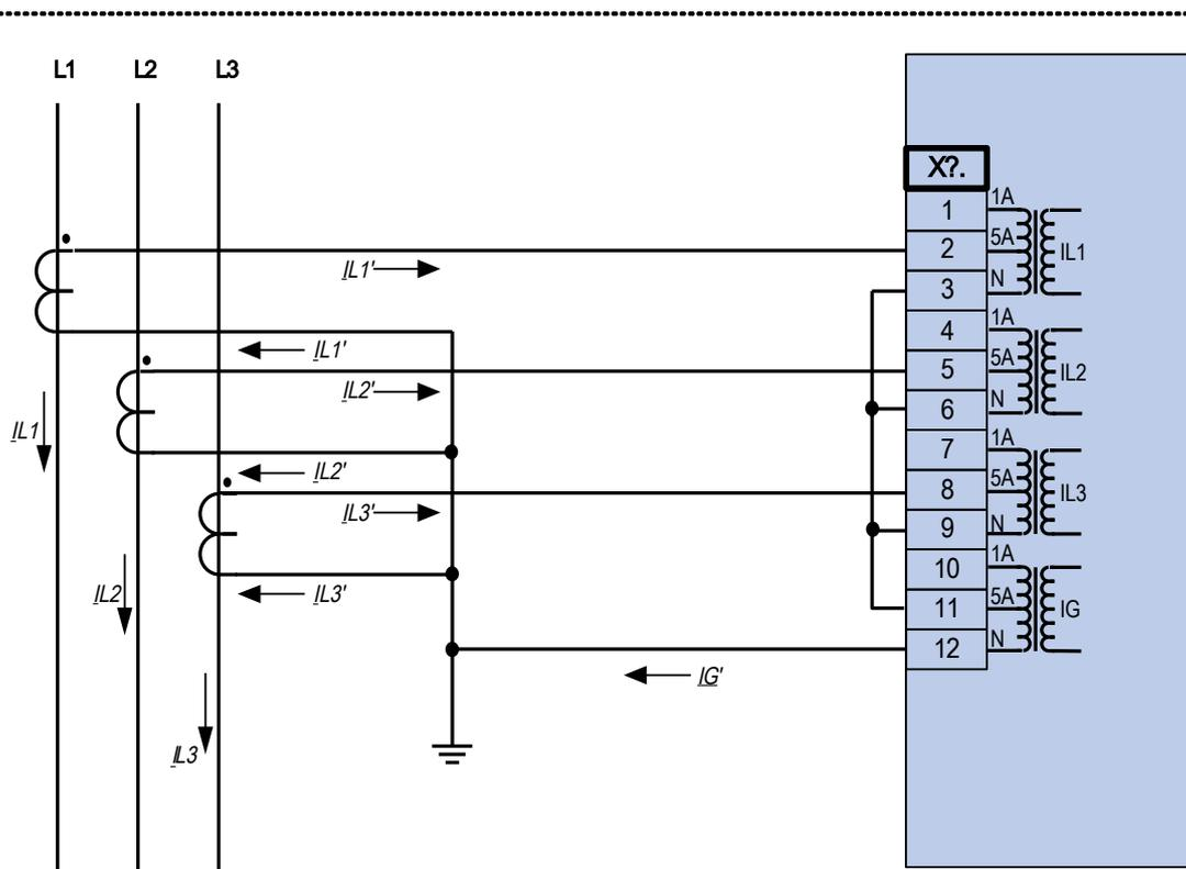
Three phase current measurement;  $I_n$  secondary = 5 A.
