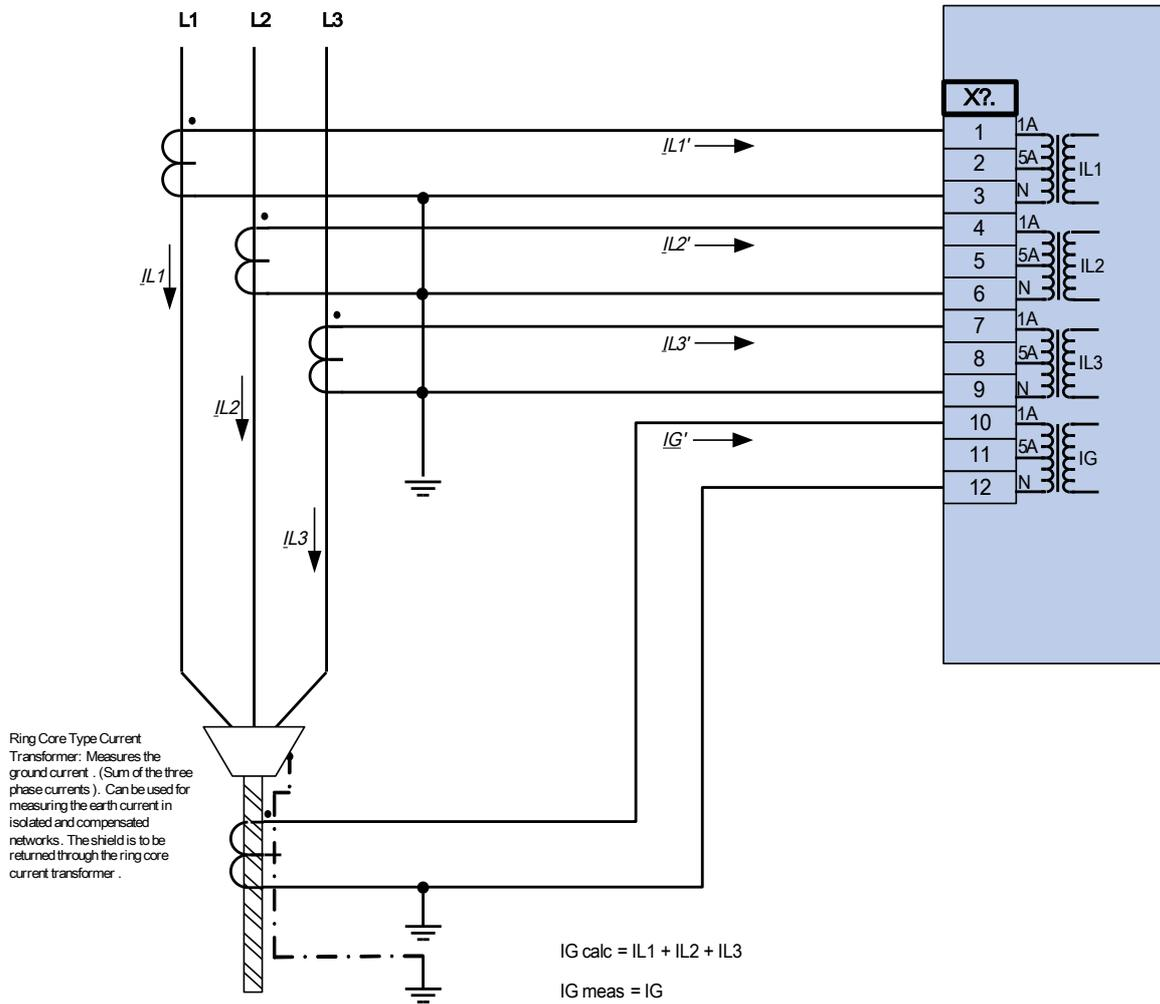
Three phase current measurement ; In secondary = 1 A.
