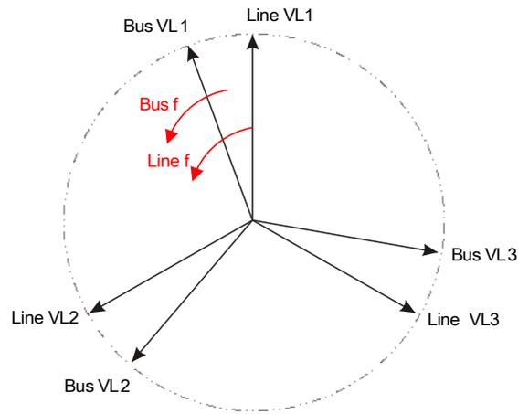
If the generator frequency  $f_{\text{Bus}}$  is not equal to the mains frequency  $f_{\text{Line}}$ , it results in a slip frequency  $\Delta F = |f_{\text{Bus}} - f_{\text{Line}}|$  between the two system frequencies.
