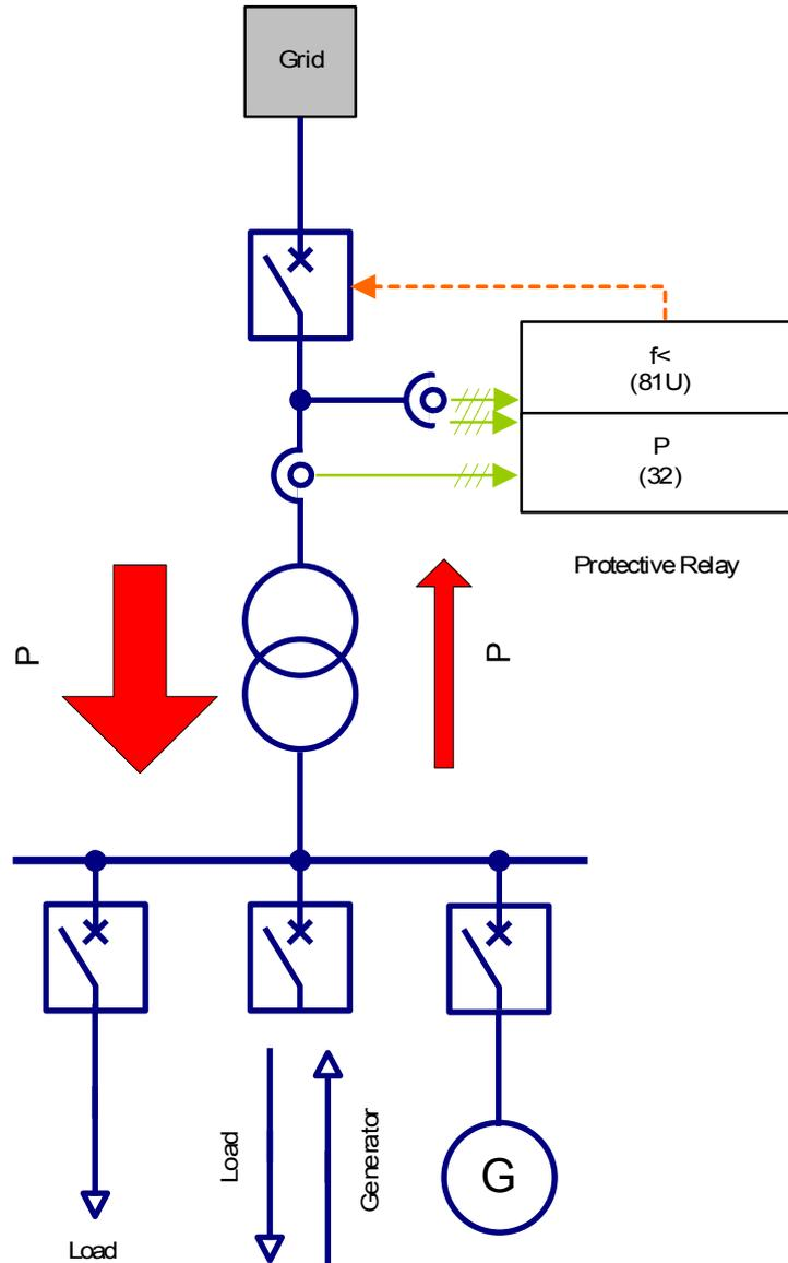
*Decentralized Under Frequency Load Shedding within grids with temporary power supply*
