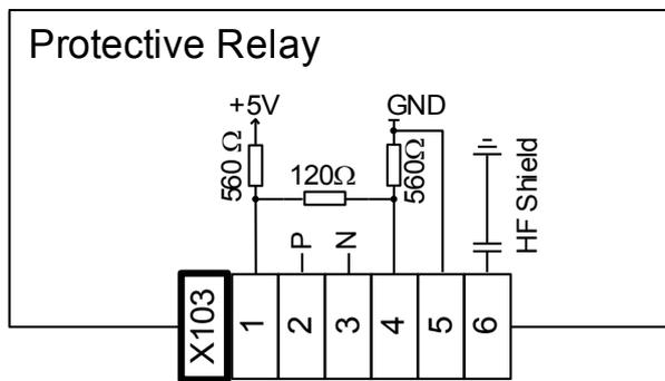
RS485 – Electro-mechanical assignment
