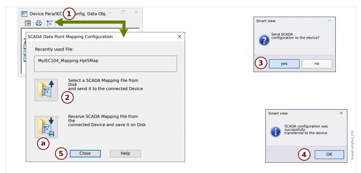
Fig. 4: Example of using Smart view to transfer the \*. HptSMap to the protection device.
