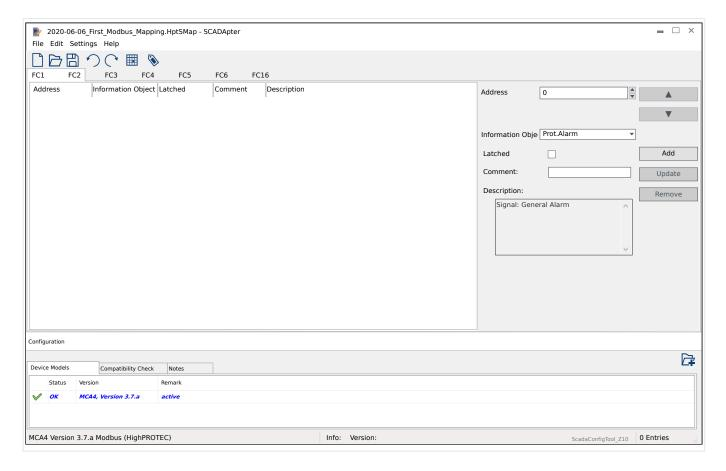
If you have selected Modbus as SCADA protocol, you can see several tabs labeled "FCx". Each of these tabs represents a Modbus Function Code and features a table that holds the mapped data objects.
