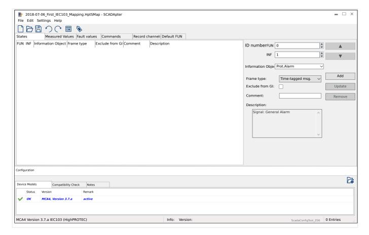
The mapping table is distributed over different tabs, representing the existing data types for the IEC 60870-5-103 protocol.
