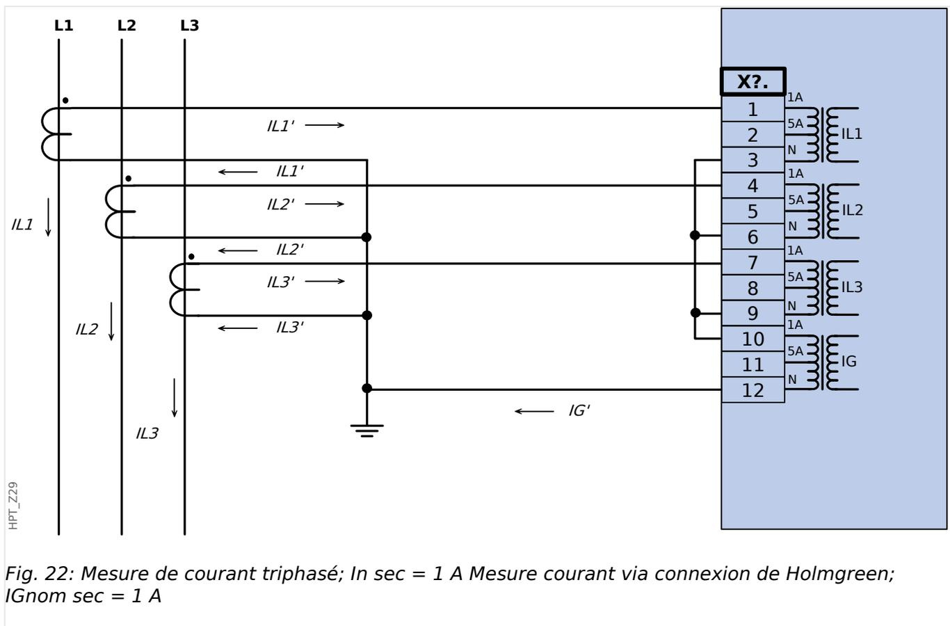
Fig. 22: Mesure de courant triphasé;  $In\ sec = 1\ A$  Mesure courant via connexion de Holmgreen;  $IGnom\ sec = 1\ A$
