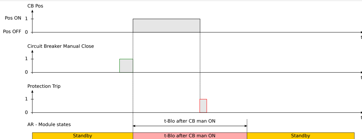
Fig. 137: Protection Trip while Manual Close Blocking time is Timing.
