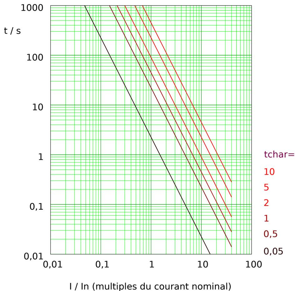
Fig. 73: I2T tripping curve. Note that only the range  $I \geq I>$  is actually effective.
