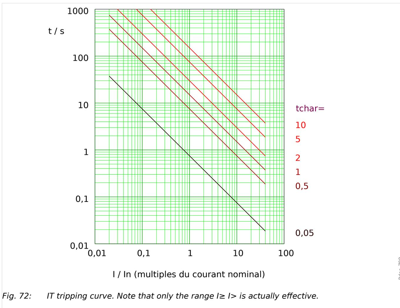
Fig. 72: IT tripping curve. Note that only the range  $I \geq I_n$  is actually effective.
