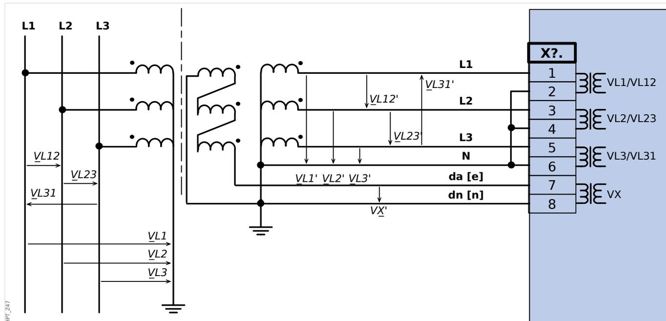
Fig. 31: VT Wye com conexão Broken Delt.
