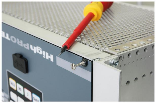
Such a 19" (sub)rack can hold up to two HighPROTEC devices of housing size B2.
