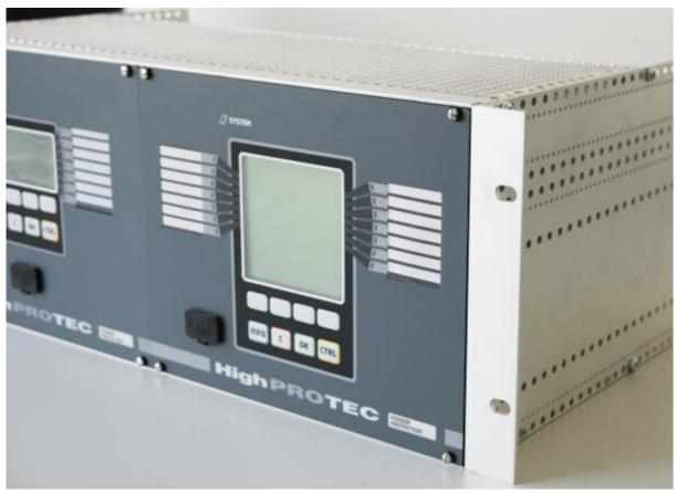
Step 6 Finally you can mount the  $19^{\prime\prime}$  rack into a cabinet in the usual way.
