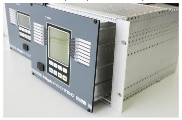
Note that the rear side of each HighPROTEC device must fit exactly between the two horizontal rails [3B], so that the device seats solidly on the lower rear rail, otherwise the mechanical stability will not be sufficient.
