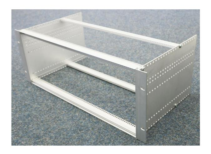
**Step 4**Use the countersunk screws [6] to fasten the small mounting blocks [7] at the cover plates [4] for the top and bottom sides.
