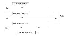
In theory the I> overcurrent and I>> short circuit function can be disabled. If the I> stage is disabled and the I>> value is set to >5x Is the earth current stage can't trip if a measured current is higher than 5x Is.
