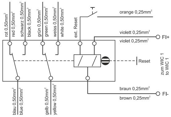
Figure 3.3: Connection diagram WI-SZ5 flag indicator
