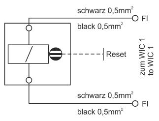
Figure 3.2: Connection diagram WI-SZ4 flag indicator
