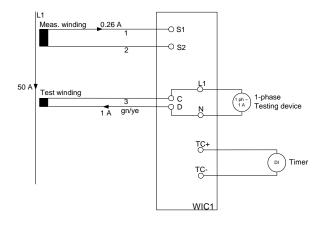
Figure 6.3: Connection of a single-phase testing device (phase L1) with CT type W2
