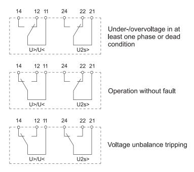
Figure 2.3: Contact positions of the output relays
