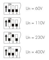
Figure 4.3: Adjustment of rated voltage
