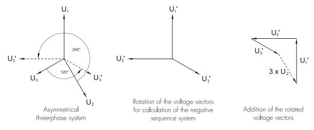
Figure 3.2: Asymmetrical three-phase system
