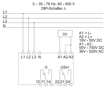
Figure 2.1: Connection three wire system
