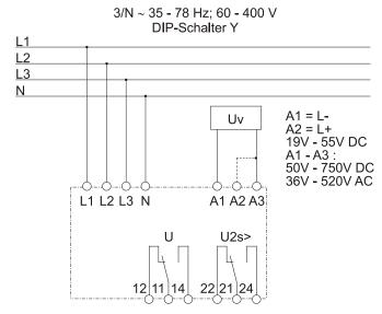
Figure 2.2: Connection four wire system
