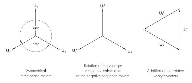
Figure 3.1: Symmetrical three-phase system
